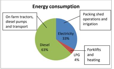
Diesel is an efficient fuel compared to petrol and LPG. Diesel engines average about 35% fuel energy conversion to work. When put through the tractor drive train, this drops to about 25%, so three quarters of the energy in the diesel is converted to heat rather than work.
