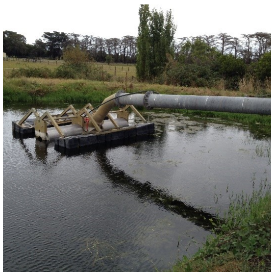
This picture shows the travelling pump intake system devised to run up and down the channel alongside the pump and boom irrigator
