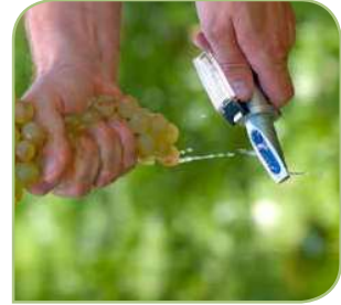
Measuring brix is vital to ensure grapes are mature and ready to eat.
