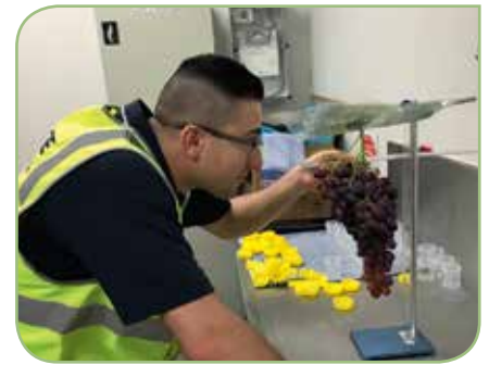
Produce Quality Inspector, Behrang Saber, measuring a bunch of Crimson Seedless grapes at the Rudge Produce Laboratory in Melbourne. Each individual berry was measured for Brix, acid, size and its 3D position in the bunch.
