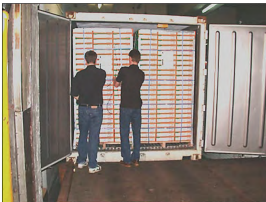
Plate 4. Sea-freight container of NZ persimmons being loaded for export. Note: ventilation spaces around the stacks of trays.
