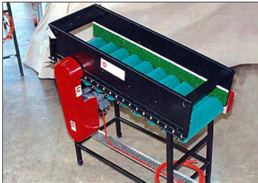
Plate 6. Polisher with several nylon brushes designed by KW engineering.
