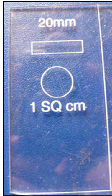
Plate 3. A simple sizing gauge to measure area of blemish.
