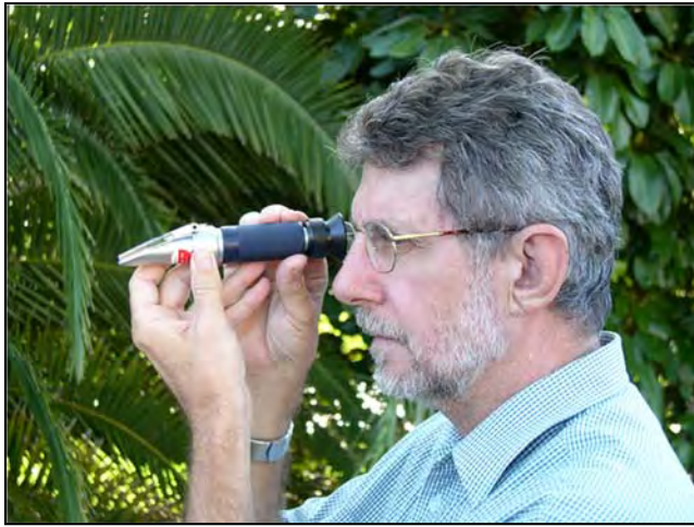
Plate 14. Left: Hand-held refractometer used for measuring sugar concentration. Right: laboratory refractometer
