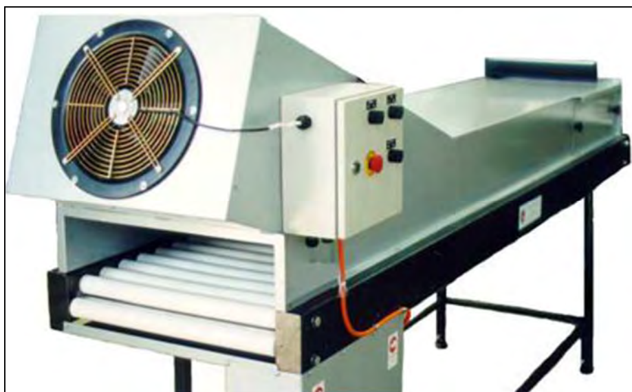
Plate 3. Drying tunnel designed by KW engineering.
