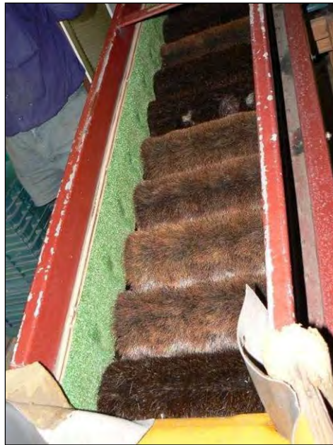
Plate 7. Rollers made of coarse horse hair about 2.5cm in length.
