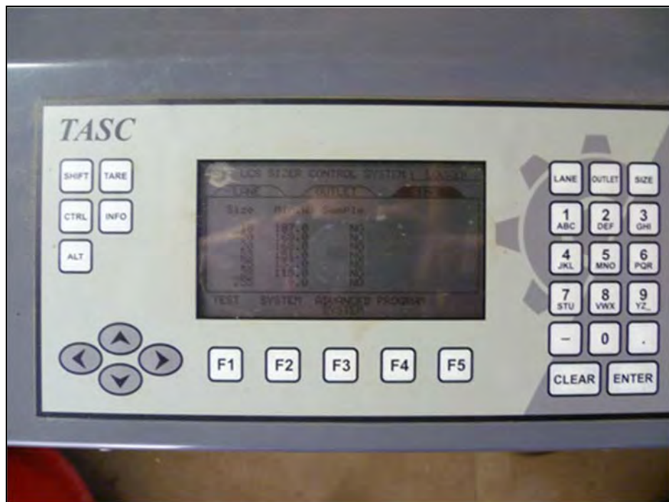
Plate 11. Electronic controllers can set weights for each size grade as well as record number of fruit packed in each size range.
