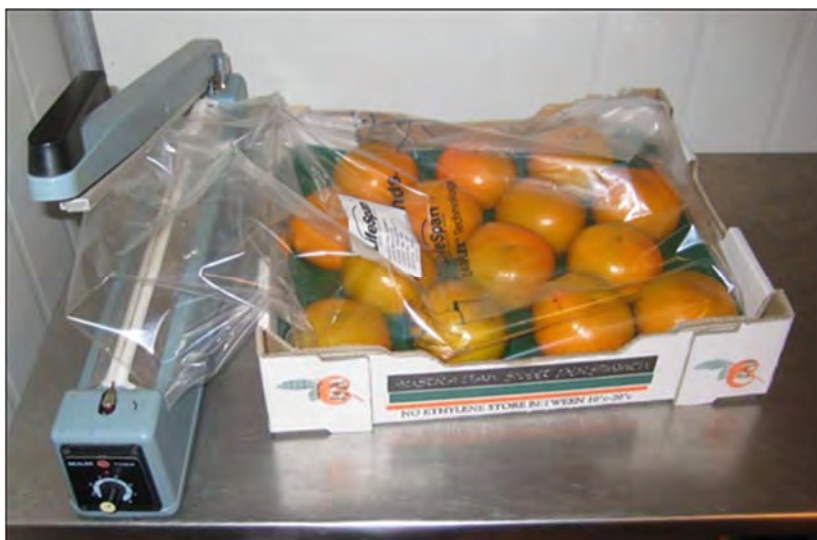
Plate 3. Fruit placed in Amcor L298 bag and heat sealed.
