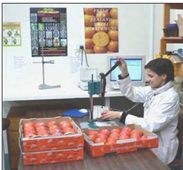
Plate 16. Testing for fruit firmness using penetrometer with 8mm head. Fruit firmness is quantified on a Shimadzu Autograph AGS-H using a 100N load cell.
