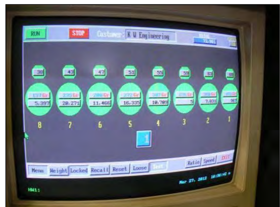
Plate 10. Electronic in-line weight grader designed by KW engineering.
