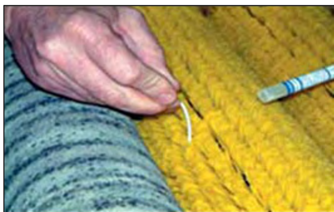
Plate 3. Swabbing wash brushes for microbial contamination. Guidelines for the Management of Microbial Food Safety in Fruit Packing Houses Bulletin 4567.
