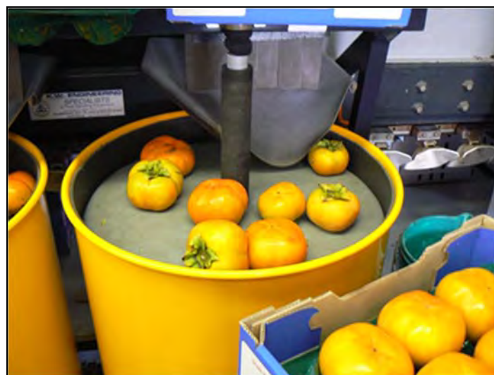
Plate 13. All bins and ramps should be padded to minimise bruising.
