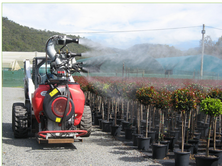
Airblast sprayers can be efficient when applying fungicides to protect large areas of high-risk crop lines. Many spray units exist for different purposes. Photo by NGIQ.
