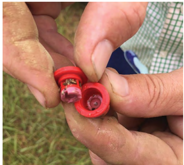
Figure 5. Regularly cleaning nozzles will improve delivery rates by removing debris build-up. Photo: Melinda Simpson.
