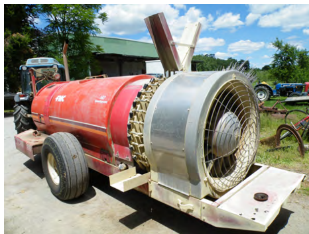
Figure 7. Deflectors on an air-blast sprayer. Photo: Sprayers 101.
