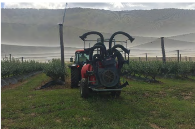
Figure 1. A ducted air sprayer. Photo: Melinda Simpson.
