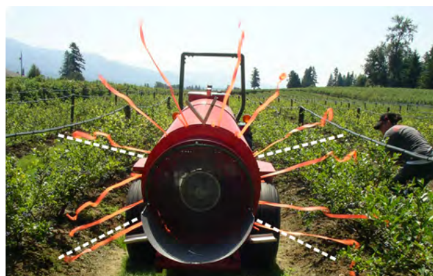
Figure 8. Using ribbons to work out where the air is being directed from the sprayer. Photo: Airblast101 Handbook.
