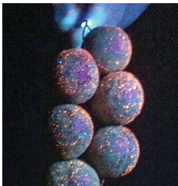
Figure 15. Using fluorescent dyes to demonstrate coverage. Photo: Jeremy Bright.
