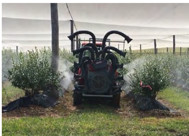
Figure 6. Assessing the sprayer output is towards the canopy. Photo: Melinda Simpson.
