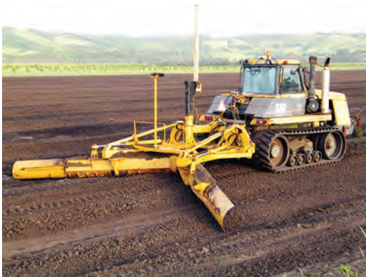
Mounding of tree rows during preplant ground preparation.
