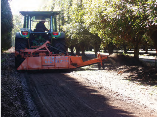
A typical soil profiler: a rotary hoe and side throw belt.
