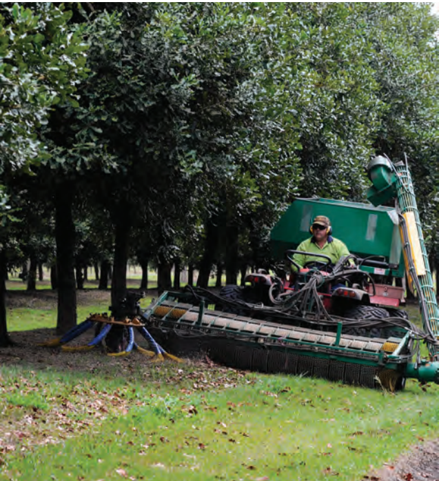
A sweeper moves less soil than a blower, but can create a depression along the drip line that may need management.
