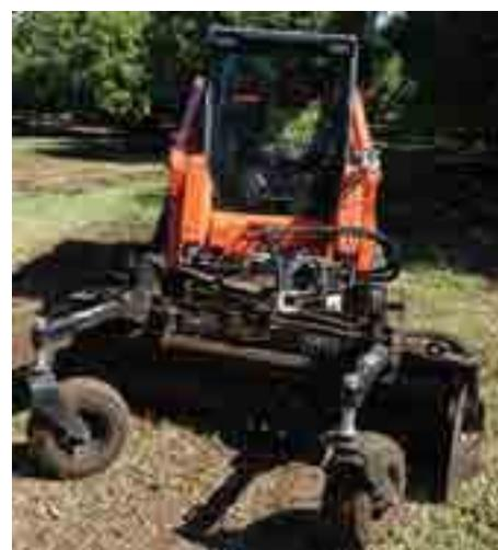
(left) Close up of the Harley rake and the skid-steer loader with the rake fitted to it.
