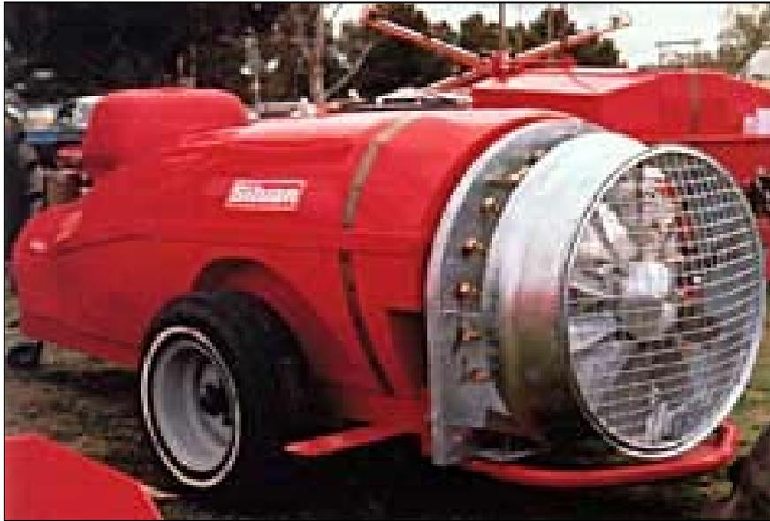
Plate 3. Low-profile air-blast sprayer.
