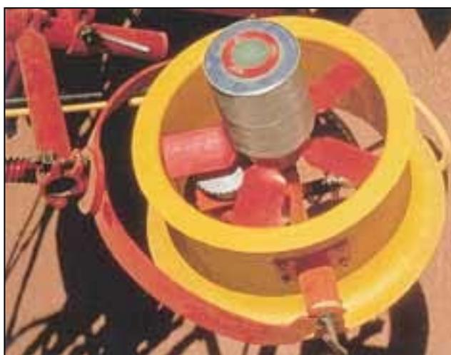
Plate 8. One type of rotary atomiser.
