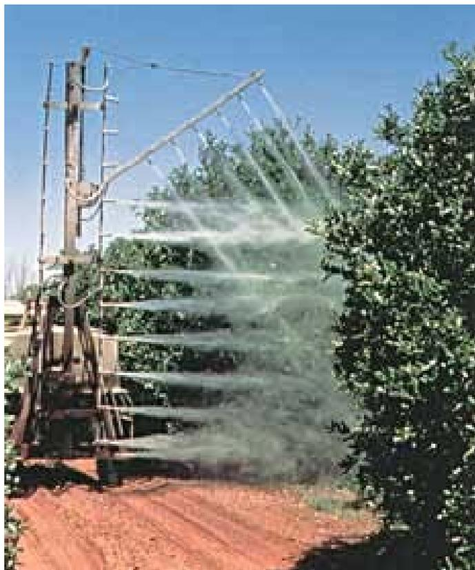
Plate 2. Oscillating boom sprayer.
