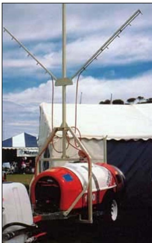
Plate 5. Structurally modified low-profile air-blast sprayers.
