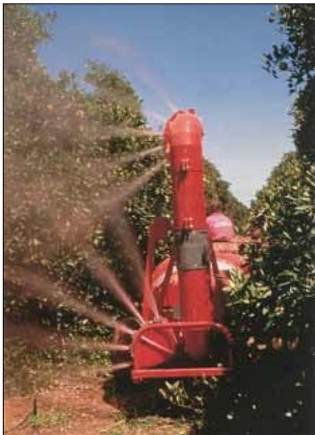
Plate 7. High-velocity air-shear sprayer with tower attachment.
