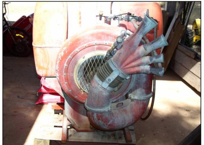
Plate 4. Different types of low-profile air-blast sprayers used by small growers.
