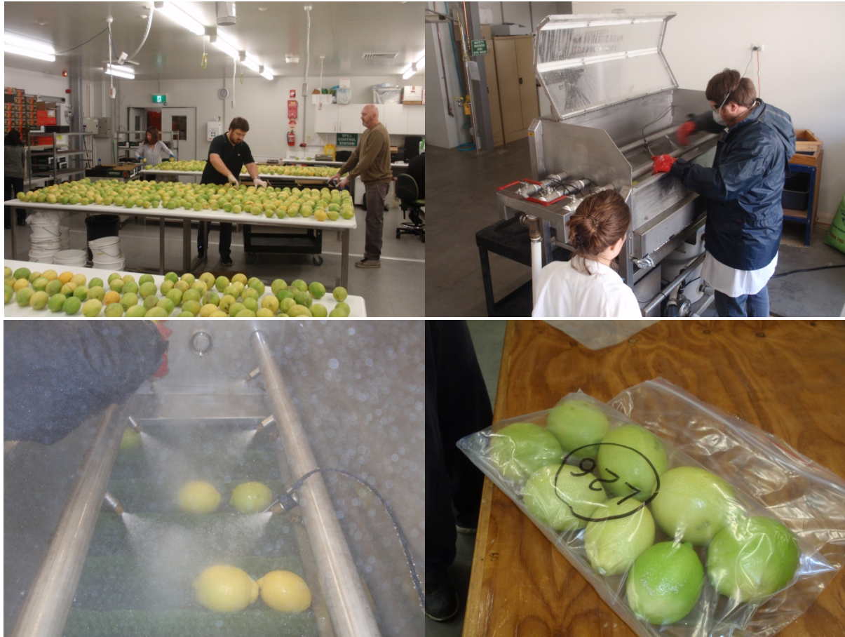
Figure 1. Lemons were randomly selected for treatment (top left), washed in a custom built experimental washing unit (top right), with brushes and high pressure nozzles (bottom left), before drying for 1 hour at 20C (bottom right) then frozen (-20C) and sent for dithiocarbamate residue analysis at Symbio Laboratories in Brisbane.
