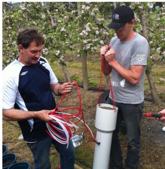
Figure 3: Installation of drainage lysimeters at Lucaston..
