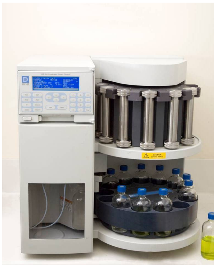
Figure 5. The Dionex Accelerated Solvent Extraction (ASE® 300) used to determine oil content in freeze-dried avocado tissue. The stainless steel cells that contain the ground avocado tissue are shown (12 per run), with the collection bottles underneath. One collection bottle is shown on the right showing the hexane/oil mix (the green pigmentation is clearly visible).
