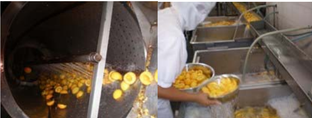
A caustic wash removes the skin before fruit is collected in basins by trimmers
