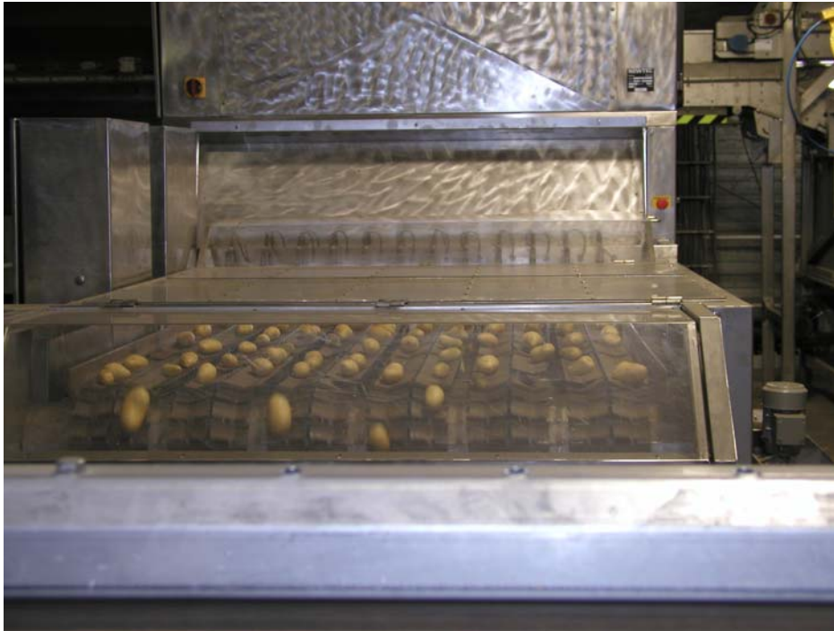
Figure 1: Infra-red machinery used to detect defects on tubers during grading process.
