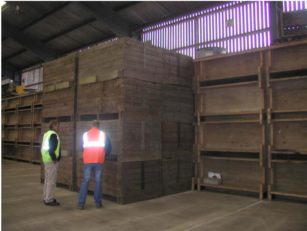
Figure 5: Letterbox system used by Grampian Growers for curing of tubers.
