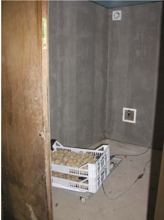
Figure 4: 'Hot Box' used to assess the potential of rot and disease development in harvested tubers.
