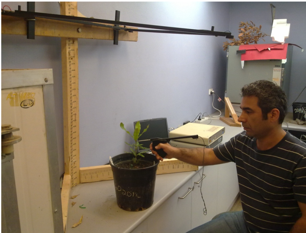
Figure 2. The set up of the digitizer: hardware, software, triangle with microphones on each corner and the pointer with trigger. When the pointer is triggered the spatial position of its tip is recorded.
