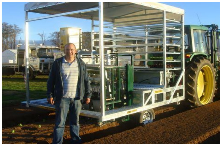
Plate 2. The Transplant Systems transplanter (for non-plastic situations.)
