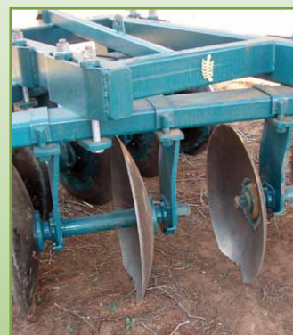
Darryl's custom-made plough to break up old plants and dig in with the soil – very heavy duty!
