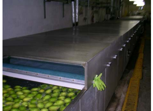
The hot and cold dips are included as part of the conveyor system at Caliman Agricola.
