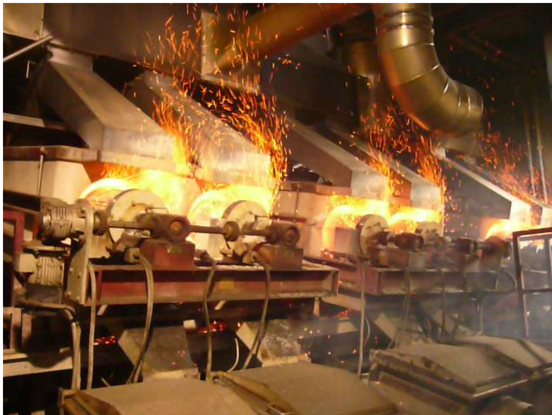
Bank of six brulage ovens – the nuts are dropped into the top of the unit. The nuts leaving the units can be seen on the conveyor belt underneath the main cylinders.
