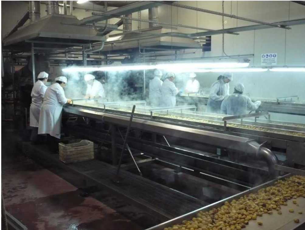
Nuts being graded after passing through the wash and brush unit. The heat from the nuts can be seen (i.e. steam) and the nuts actually end up being semi-cooked in this process.
