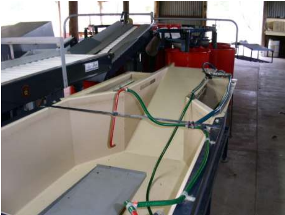
Figure 1. Harvested fruit placed into tank. Water flow is used to carry fruit to rollers.
