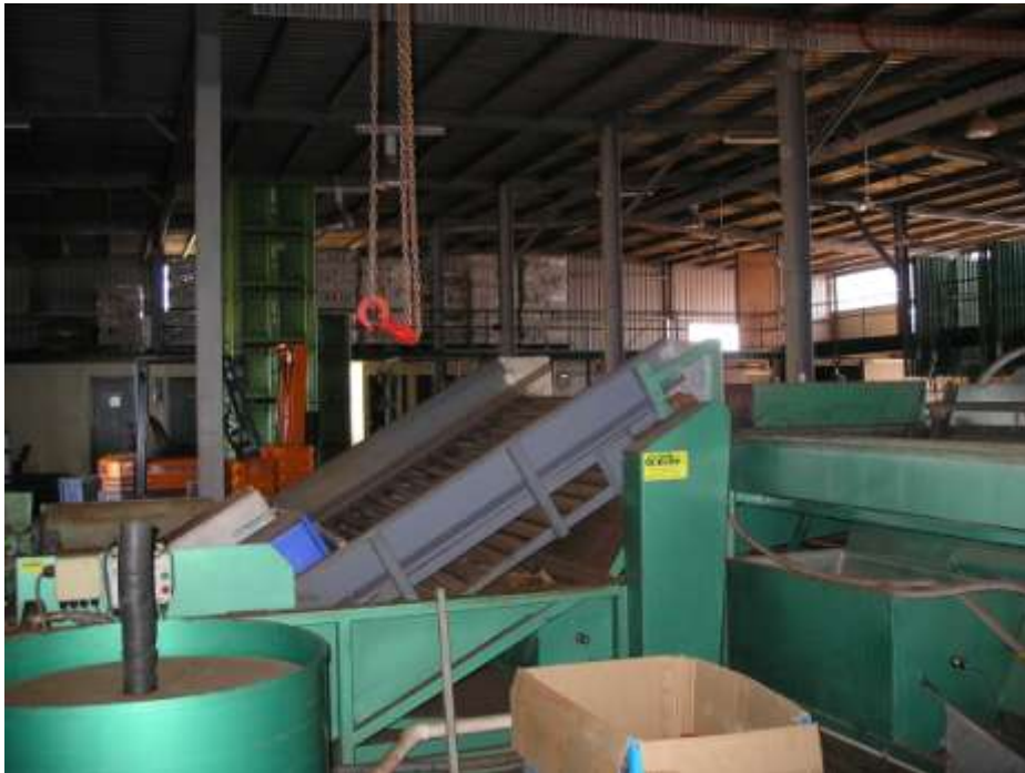
Figure 6. Fruit is then deposited into a fungicide dip. The scoops move the fruit through the dip (in the direction of the arrow).
