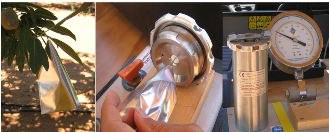
**Figure 1.4:** Pressure bomb assembly to measure stem water potential.
