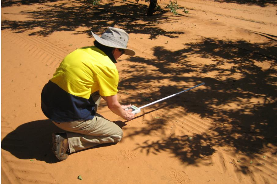
**Figure 1.2:** Light interception measurement using a ceptometer.
