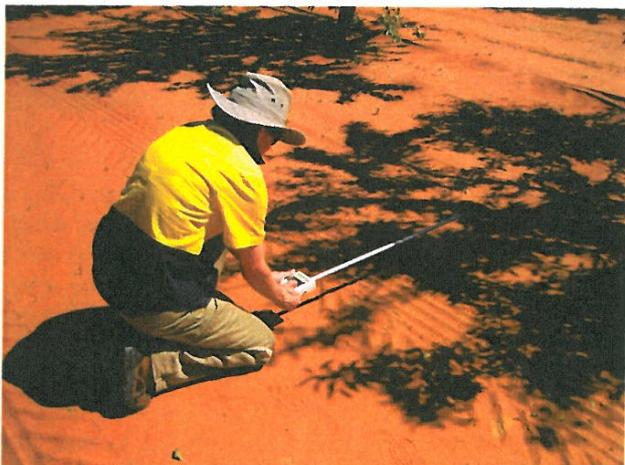
Figure 1. Light interception measurement using a ceptometer.
