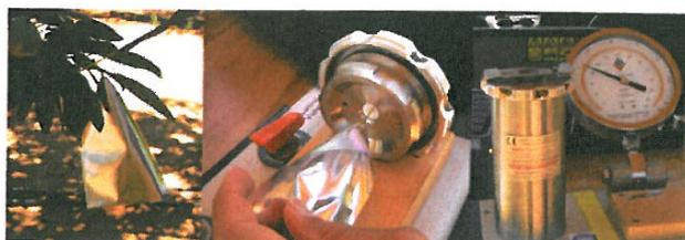
Figure 3: Pressure bomb assembly to measure stem water potential.
