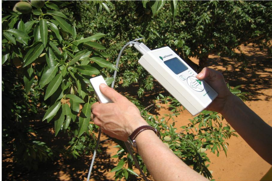
**Figure 1.3:** Stomatal conductance ( $g_s$ ) measurement using a Decagon leaf porometer.
