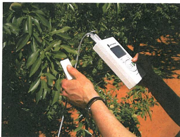
Figure 2. Stomatal conductance measurement using a leaf porometer.
