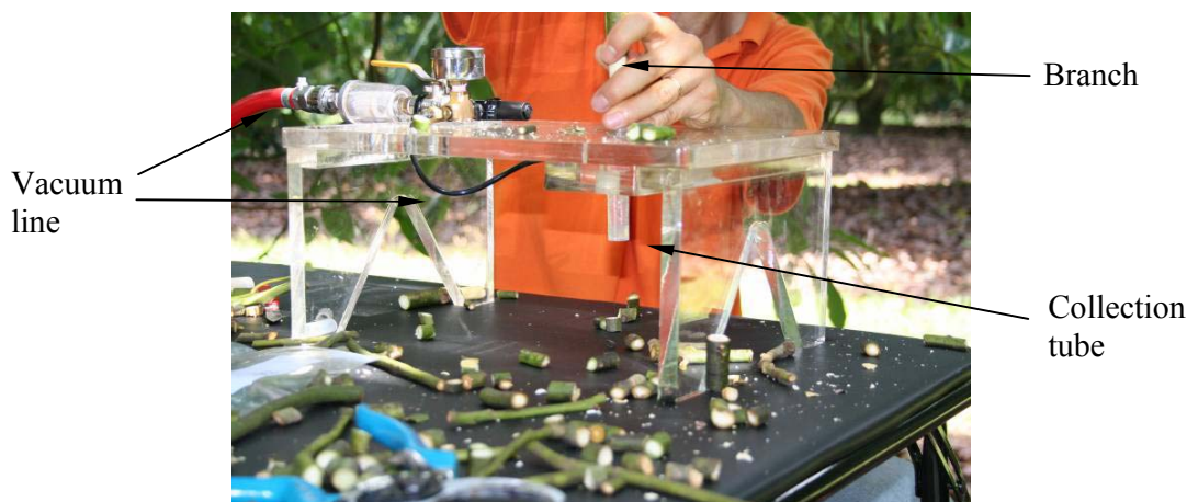
Plate 1. Equipment used to extract xylem sap under vacuum from small Hass avocado branches.
