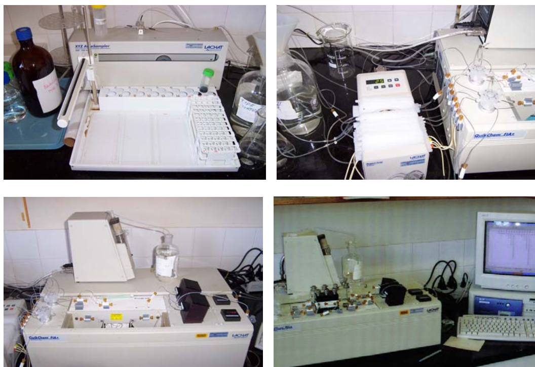
Figure 4 Flow Injection Analyser (FIA) used for pyruvate measurement at NSW DPI Wagga Wagga Agricultural Institute
