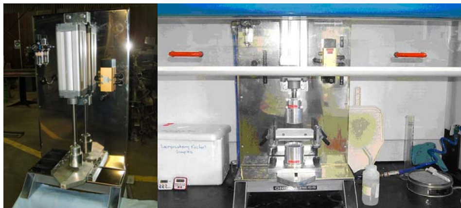
Figure 2 Onion press designs and operating press at NSW Department of Primary Industries, Wagga Wagga Agricultural Institute
