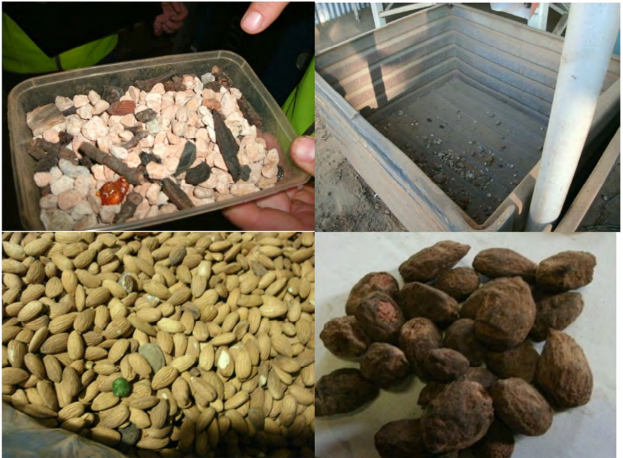
Figure 2.17 Foreign matter removed by a laser sorter at the packers (top left); stones removed by a destoner machine at Costa Almonds (top right); tiny green melons in the product from the hullers and shellers (bottom left); dried peaches removed from almonds at hulling and shelling stage (bottom right).
