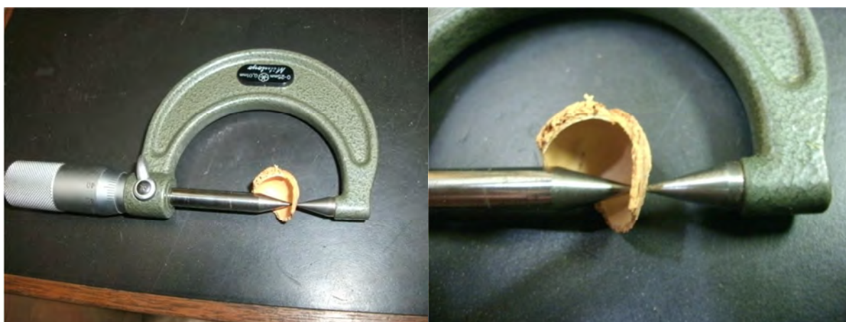
Figure 4.15 Measuring the thickness of the almond shell with a point micrometer.
