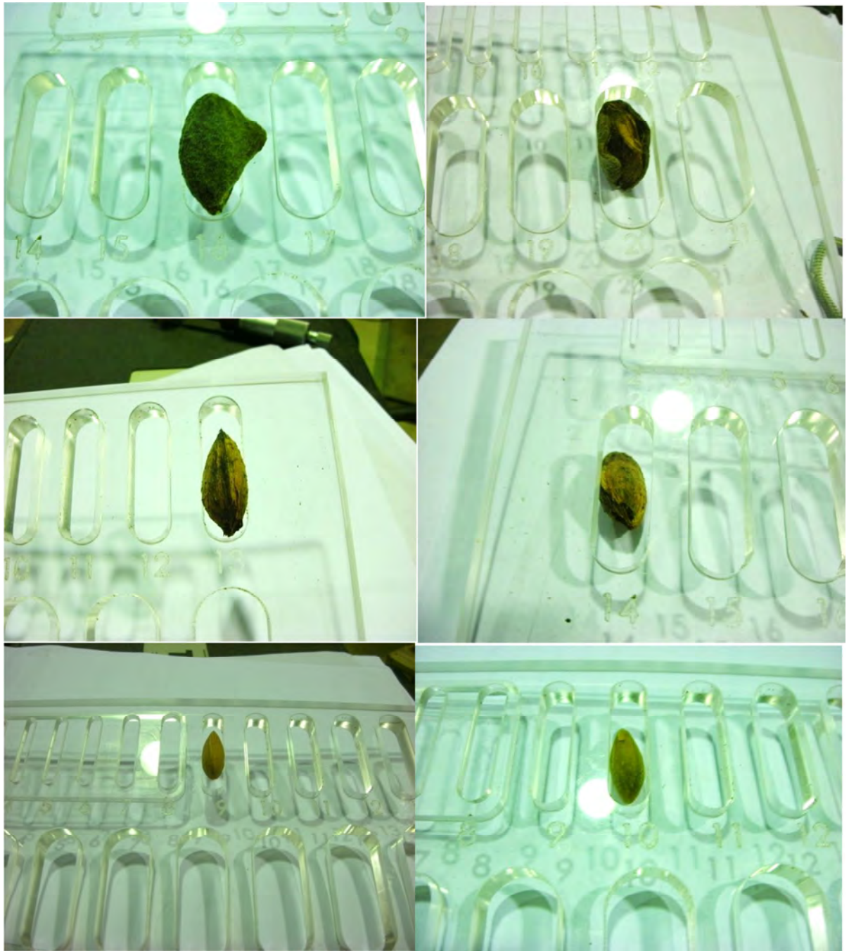
Figure 4.3 Top row, grading the in husk almonds by thickness. Middle row, grading the in-shell almonds by thickness. Bottom row, grading the kernels by thickness.
