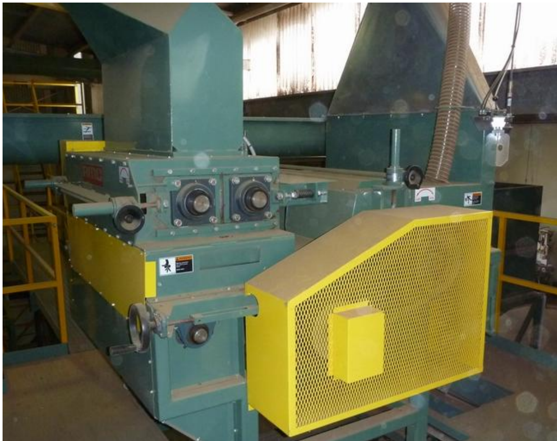
Hulling and shelling is undertaken using shear rollers (upper) and a shear roller running over a belt (lower).
