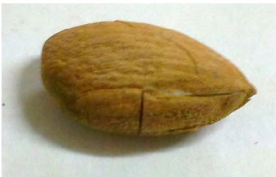
Figure 5.5 Almond with obvious crack after impact by steel anvil.
