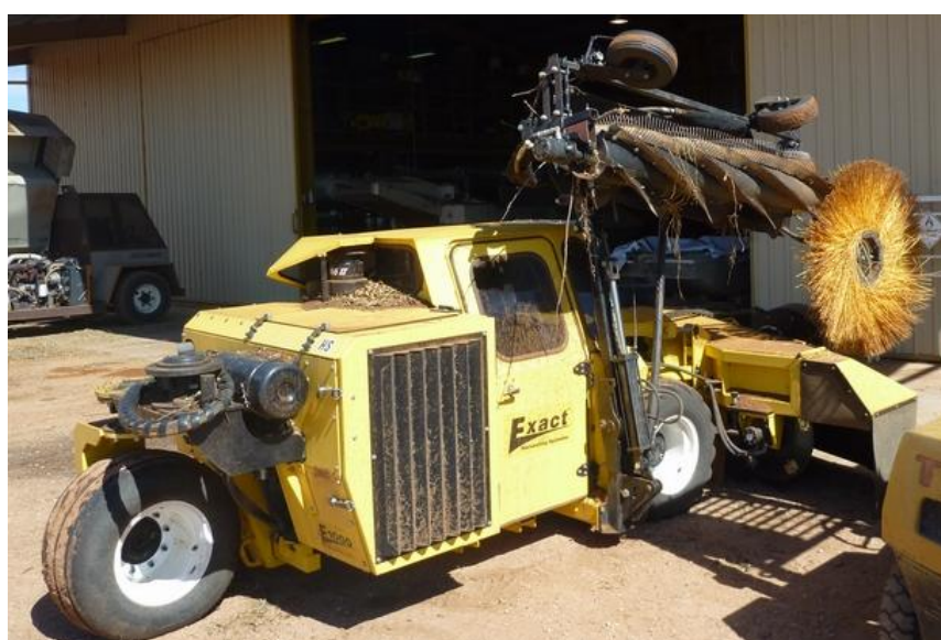
A new style (Exact) sweeper has an additional rotary brush to help gather kernels. One of the 2 brushes was removed as it was too difficult for the operator to control.
