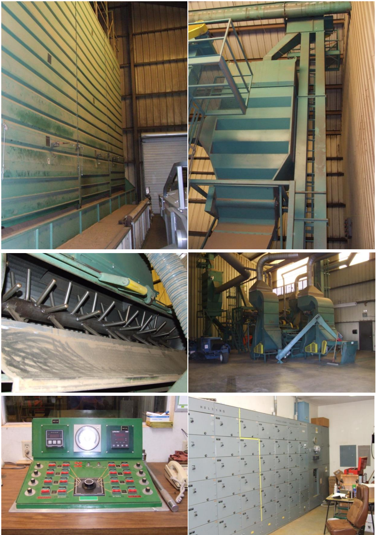
Figure 16: Montgomery's bulk drying facility, clockwise from top left – pre-cleaner, central boiler, heat exchange (water pipes, radiators and fans), silos, vented cooling tower, pin roller, hulling line, control panel, and power boards.
