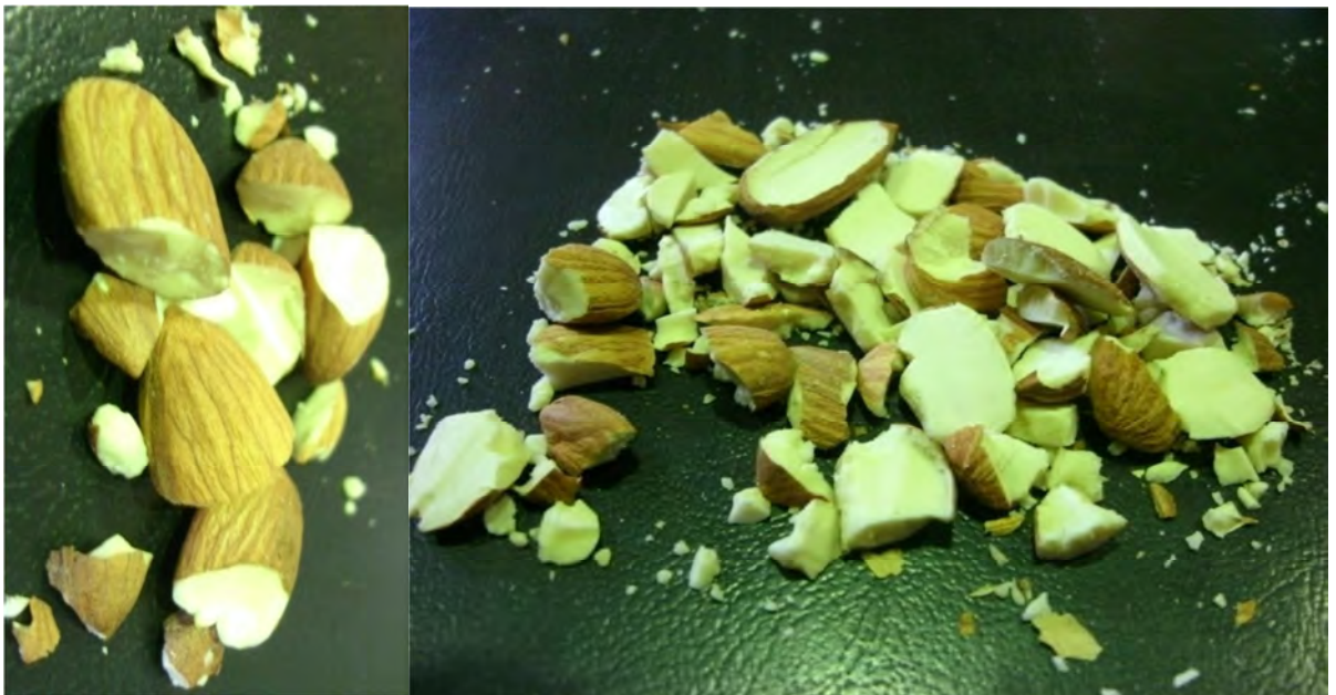
Figure 5.13 Almond kernels broken into pieces at 13 m/s (left) and 24.8 m/s
