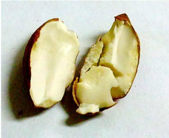
Figure 5.3 Almond kernel that was broken by the anvil of the pendulum impact tester.
