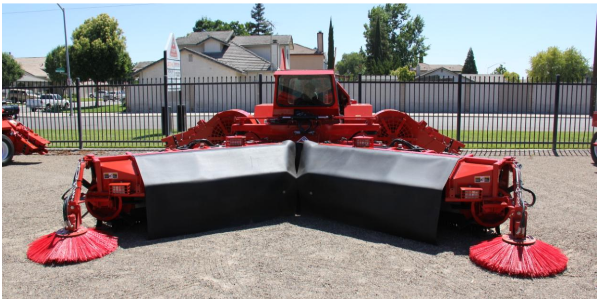
Figure 13: Flory Industries, Flory Super V60 Series, doubled sided sweeper.
