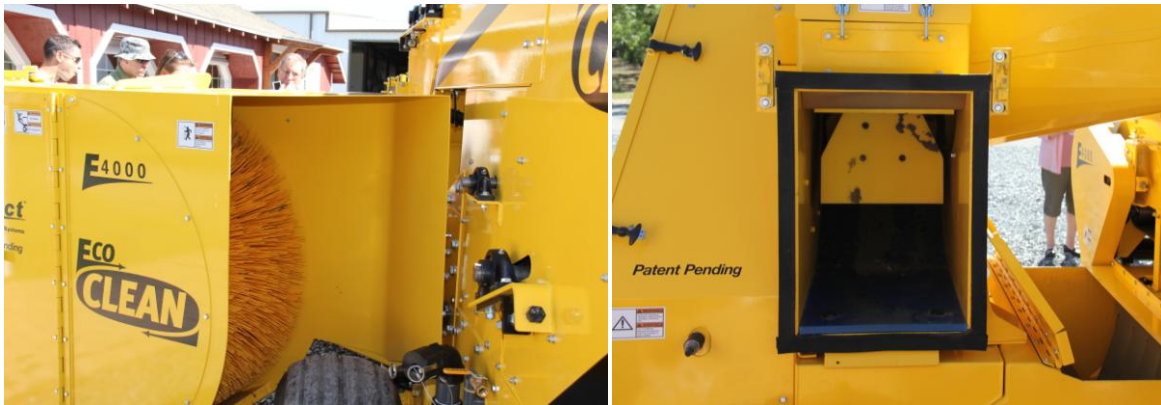
Figure 14: Exact Harvesting Systems, E-4000 Eco-Clean dust minimisation system. Left picture indicates the mechanism for wetting the soil and the brush to dispose of the wet soil. The right photo indicates the shoot for the debris disposal following the air lock mechanism.
