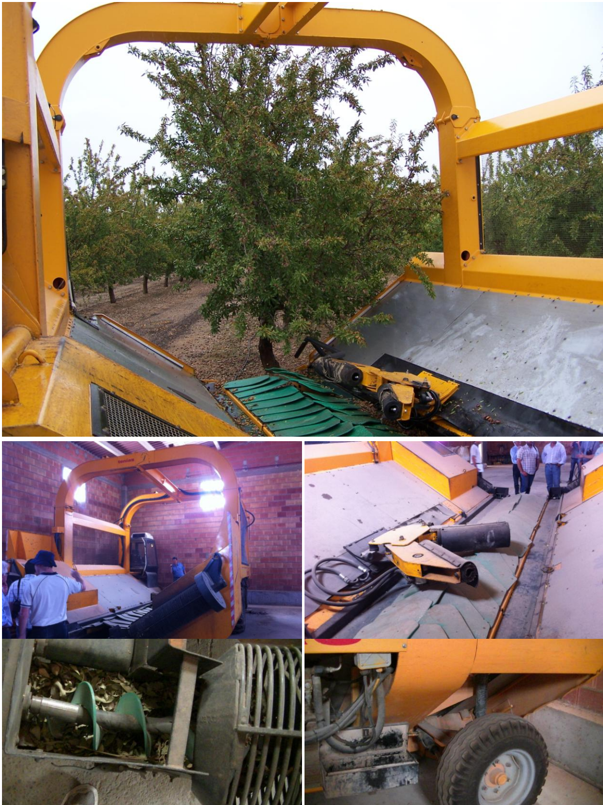
Figure 10: Tenias, over the row, continuous moving almond harvester, Spain.
