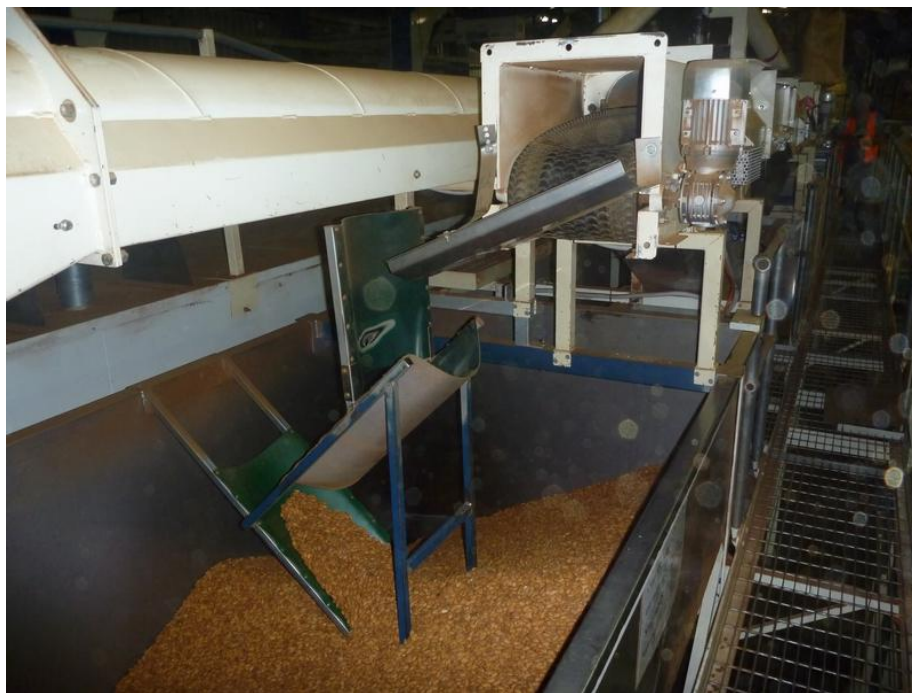
Cascades to reduce damage to falling almonds.
