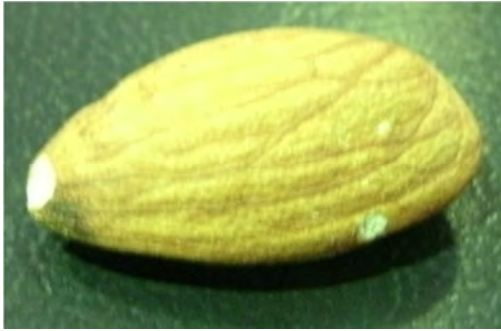
Figure 5.11 Almond kernel Chipped at 5.5 m/s velocity.
