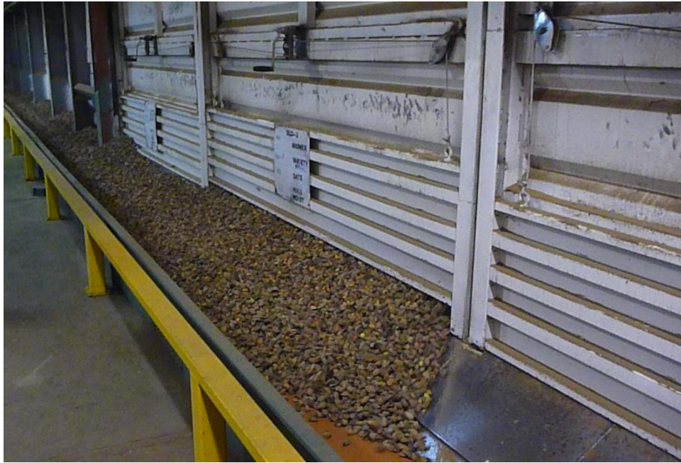
The flow from the silo is regulated by the gate height.
