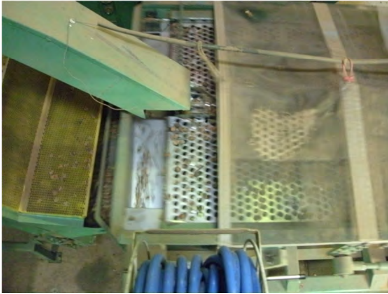
Figure 2.12 Vibrating screens with round holes separate kernels from husk and shell remnants
