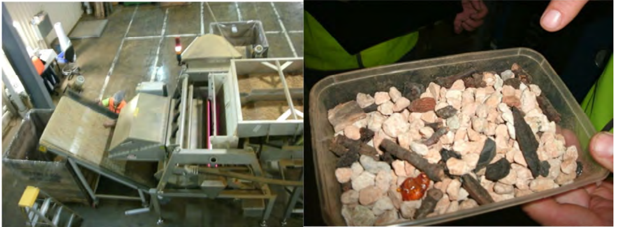
Figure 3.3 Riverland Almonds' laser sorter (left) removes foreign material (right).
