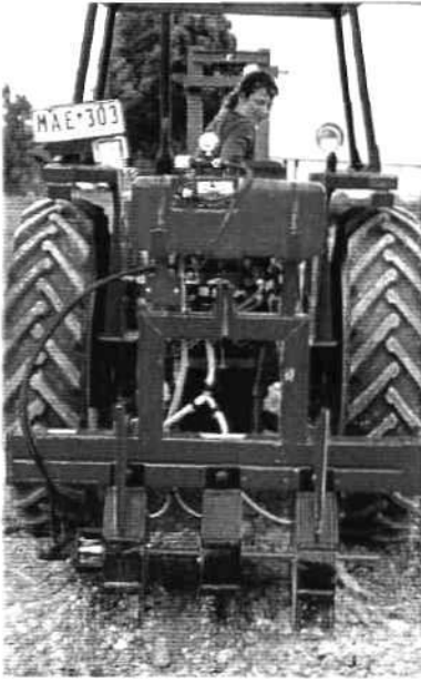
Figure 16: Precision incorporation machines designed to incorporate products into the transplant rows for improved clubroot control. A) Victorian machine designed to operate between tractor and transplanter for single pass operation B) NSW machine.
