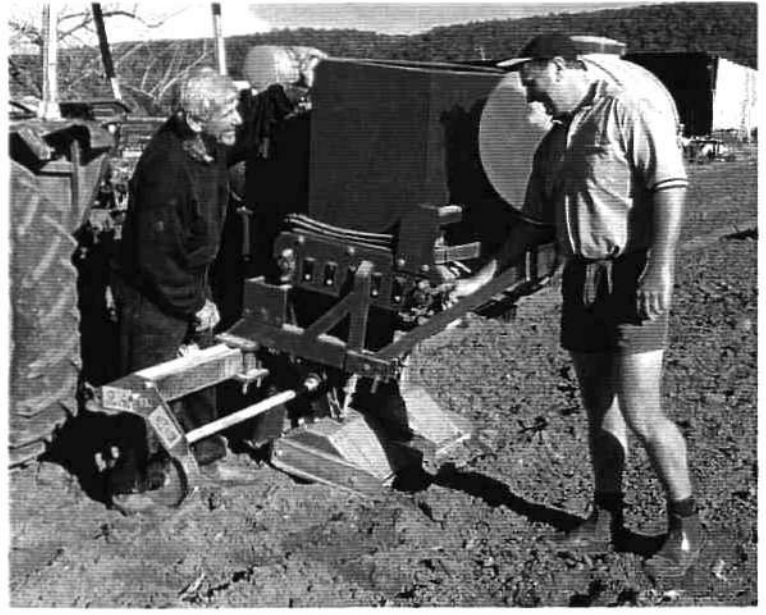
Figure 16: Precision incorporation machines designed to incorporate products into the transplant rows for improved clubroot control. A) Victorian machine designed to operate between tractor and transplanter for single pass operation B) NSW machine.
