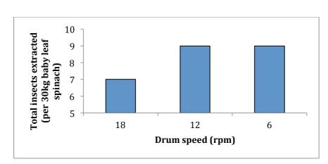
Figure 61 Impact of drum speed on the removal of insect contaminants from baby leaf spinach
