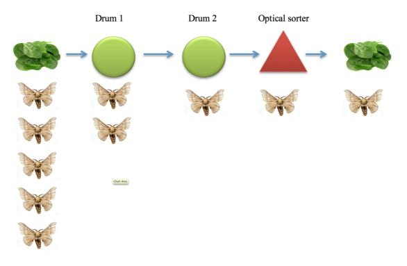
Figure 65 Schematic of the points in the processing line where insects can be removed.
