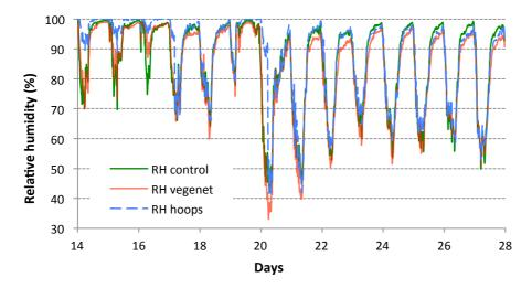
Figure 47 Relative humidity (% RH) recorded between April 2 and 16 in an open field, under VegeNet and under hoops with InsectNet
