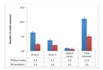
Figure 66 Number of dead or living moths out of a total of 15 removed at each stage of the processing line.
