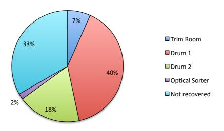
Figure 64 The efficiency of each control point in the processing line of removing Heliothis insects from spinach. Data shows % of insects removed at each point.
