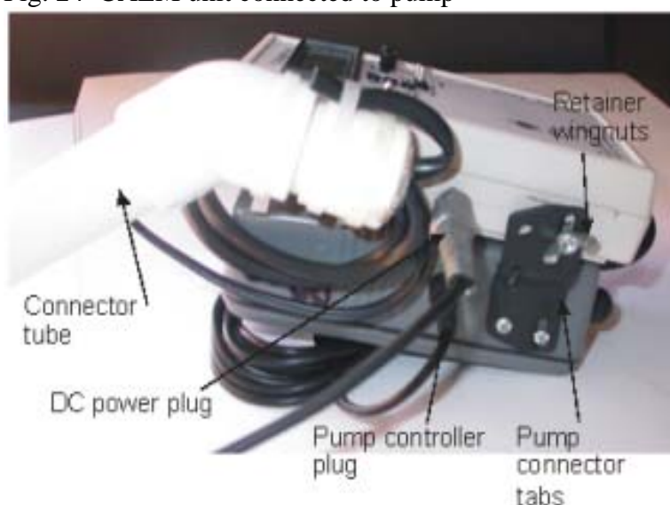
Fig. 24 CALM unit connected to pump
