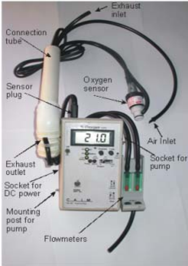
Fig. 22 Strawberry CALM unit without pump attached.
