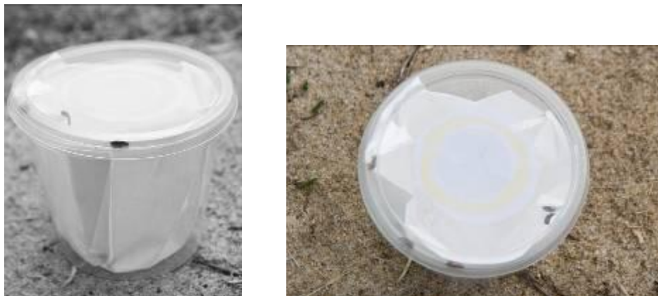
Figure 1: Cage design for acute toxicity bioassays. Cup-shaped filter papers were fitted into plastic cups (left) with ventilated lids (right).
