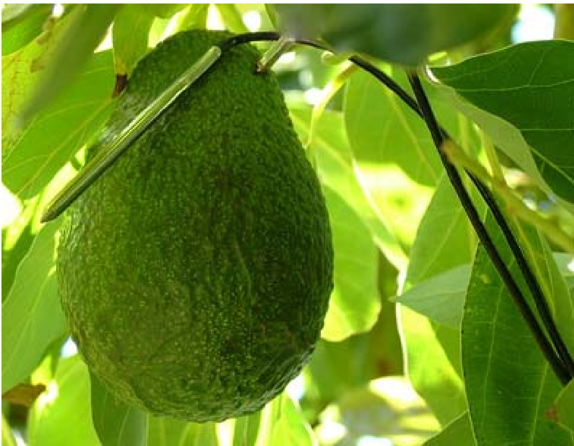
Picture 1. Probe set in avocado fruit using Cox tracer loggers fitted with twin external probes, one probe inserted into the fruit for pulp temperature readings, the other to measure ambient shaded temperature
