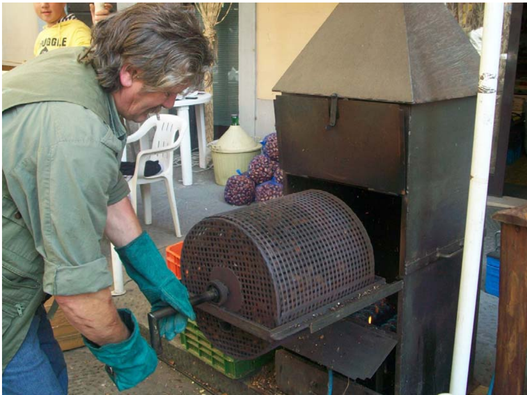
This roaster was gas fired and was a kind of combination of the tumble roaster and an oven.
