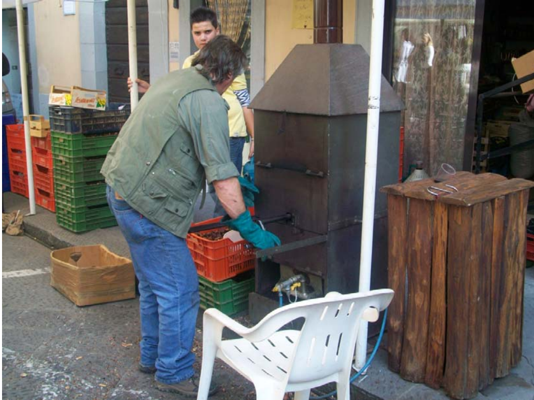
This roaster was gas fired and was a kind of combination of the tumble roaster and an oven.
