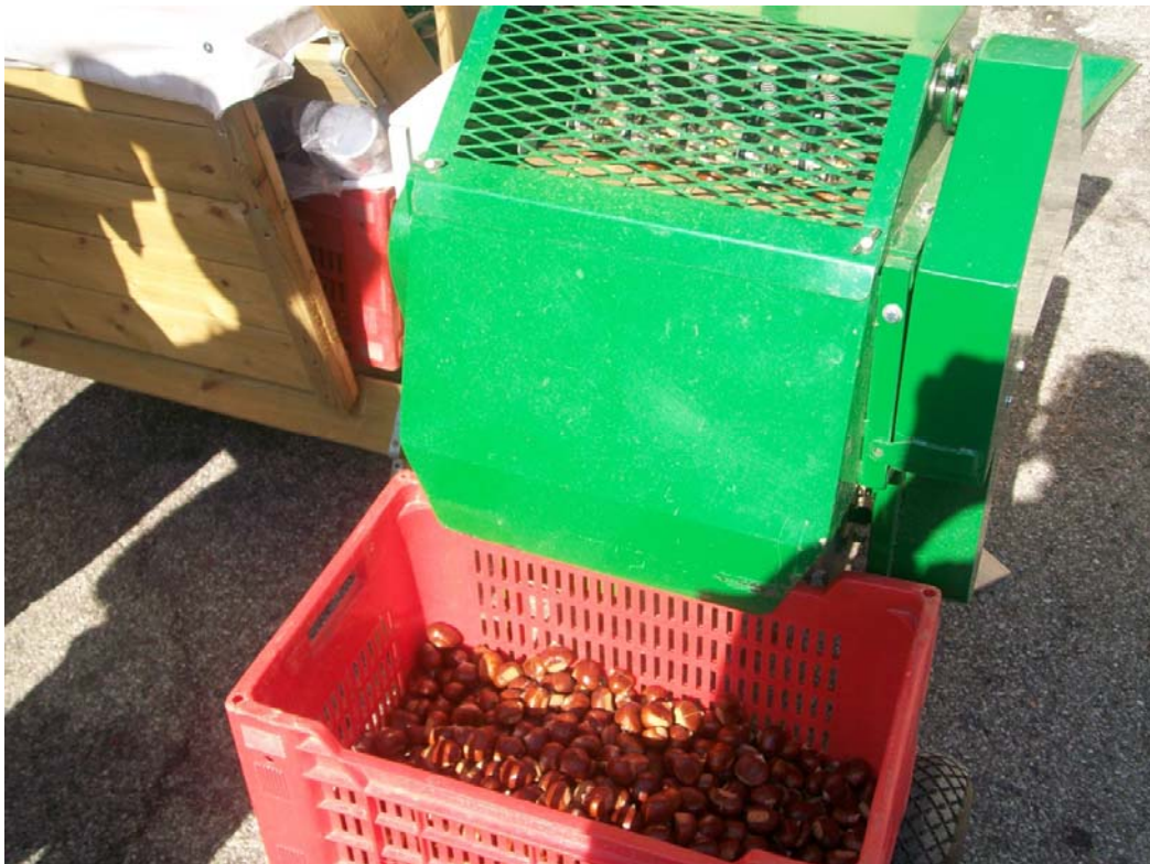
A machine for 'marking' the chestnuts before roasting – five nuts at a time.
