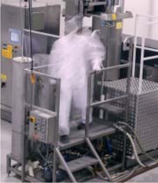
Figure 5: CSIRO's High Pressure Processing pilot plant.
