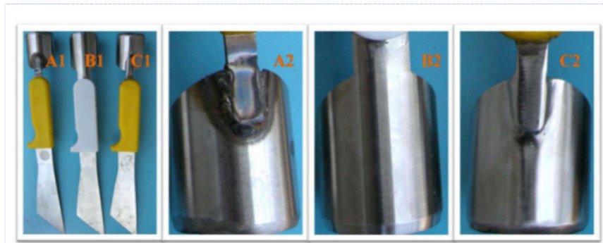
Figure 10. Development of prototype coring knife with improved food safety feature. A1: Coring knife currently widely used in the industry. A2: Enlarged image showing the rough welding of the coring ring B1: Prototype 1 – No-joint (one piece) design; B2: enlarged image showing no welding point C1: Prototype 2. Current coring knife with rough welding point polished; C2: enlarged image showing the smooth welding pint.
