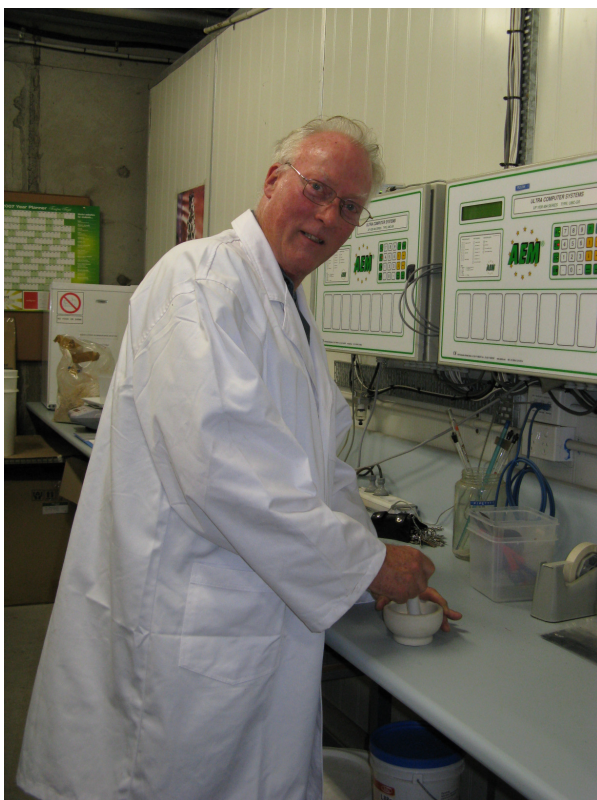
Fig 3 Alan Clift using a mortar and pestle to evenly mix imazalil granules with gypsum to treat grain spawn prior to use in laboratory evaluation as a spawn treatment.
