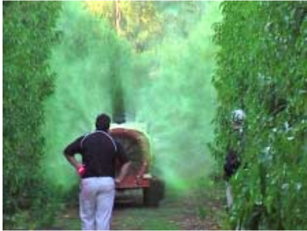
Figure 3: Water containing fluorescent dye is applied to stone fruit trees by one of the air blast spray units.
