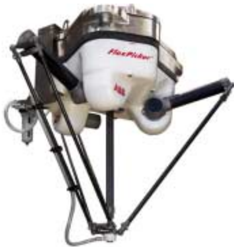
Figure 5: The ABB Flexpicker robotic arm. Figure 6: The Flexpicker on a Kiwifruit packing line.
