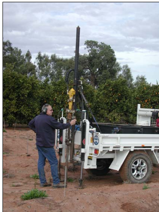
Figure 9. Deep soil samples collected between rows by a pneumatic 'hammer' corer
