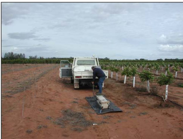
Figure 8. EM38 data collection instrument pulled between mounded rows
