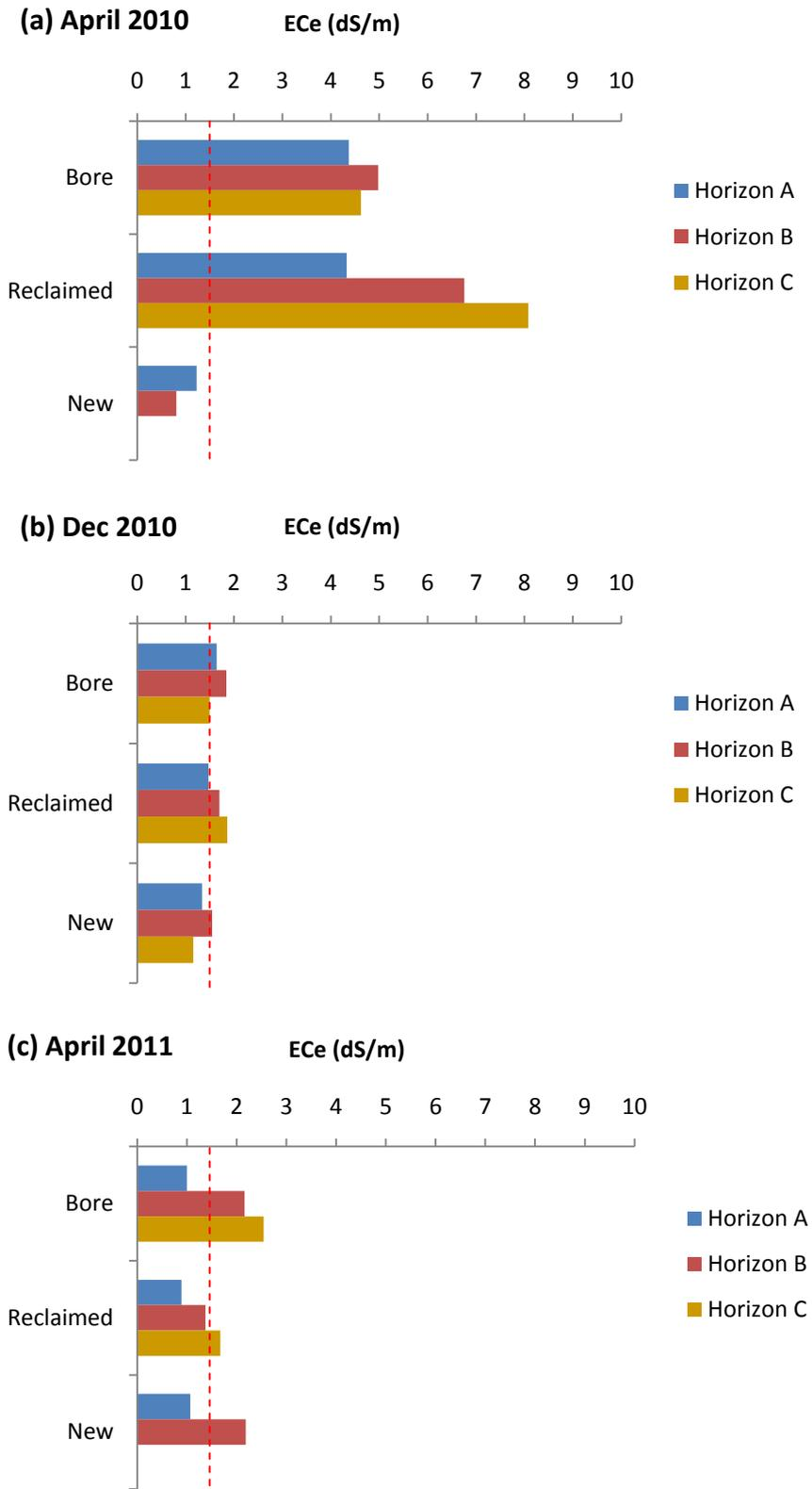
**Figure 12.** Soil salinity ( $EC_{se}$  dS/m) down a soil profile (Horizon A – C) across one year (2010/2011) at site AL2 under trees irrigated by bore or reclaimed water. The critical  $EC_{se}$  value for almonds above which yield loss occurs is 1.5 dS/m.
