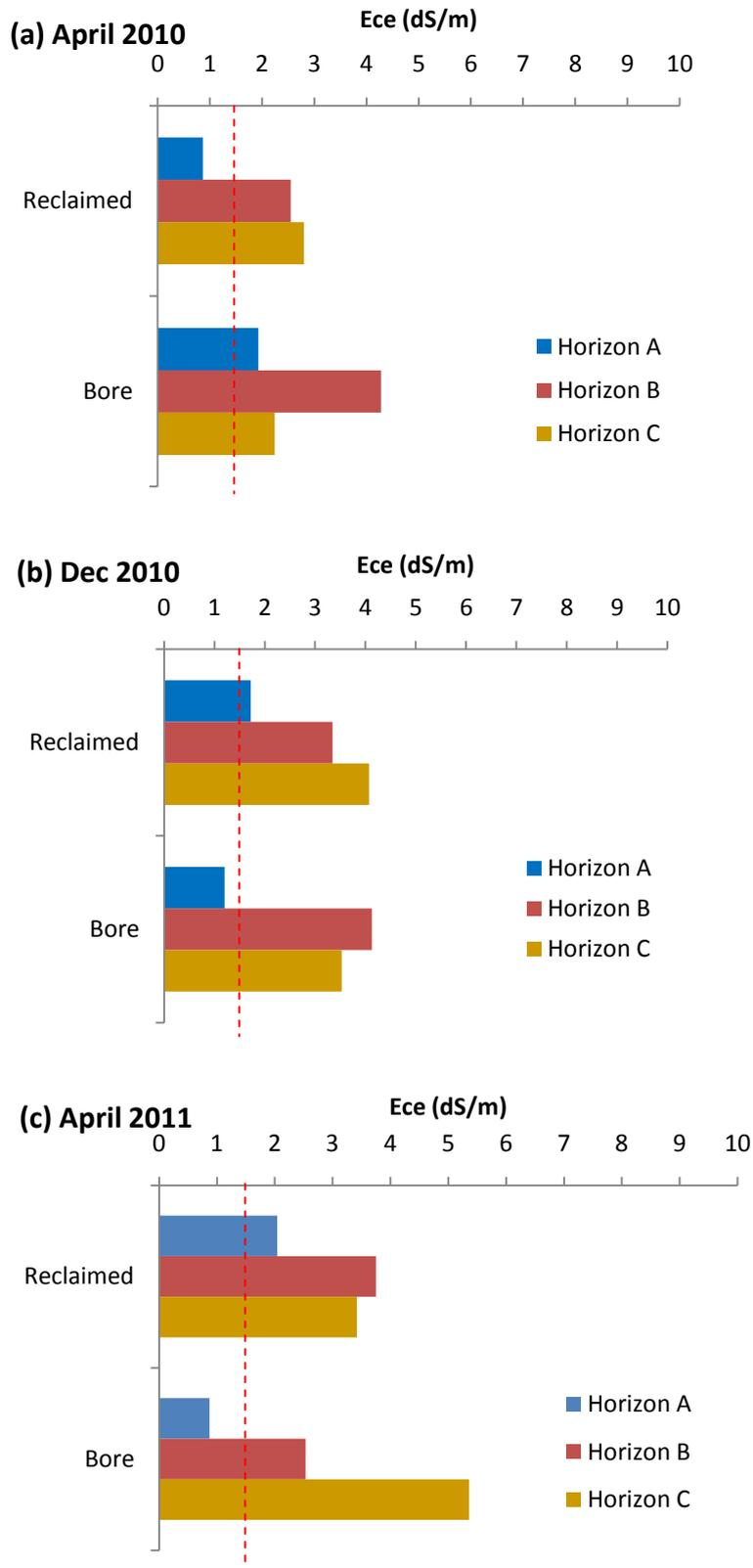
**Figure 13.** Soil salinity ( $EC_{se}$  dS/m) down a soil profile (Horizon A –C) across one year (2010/2011) at site AL3 under trees irrigated by bore or reclaimed water. The critical  $EC_{se}$  value for almonds above which yield loss occurs is 1.5 dS/m.
