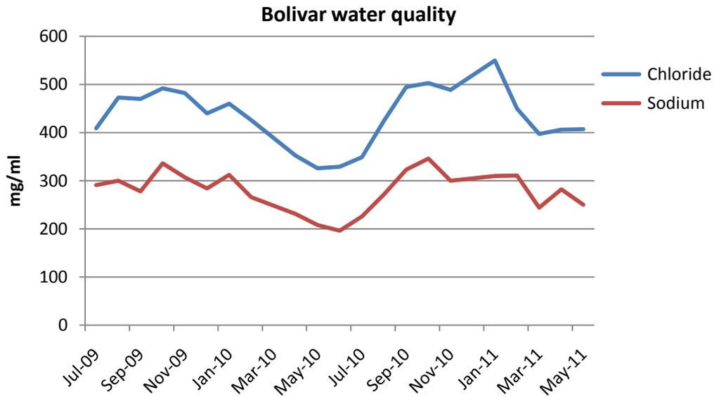
**Figure 8.** Trends in the concentration of chloride and sodium (mg/L) of reclaimed water at Bolivar wastewater treatment plant, July 2009 – May 2011.
