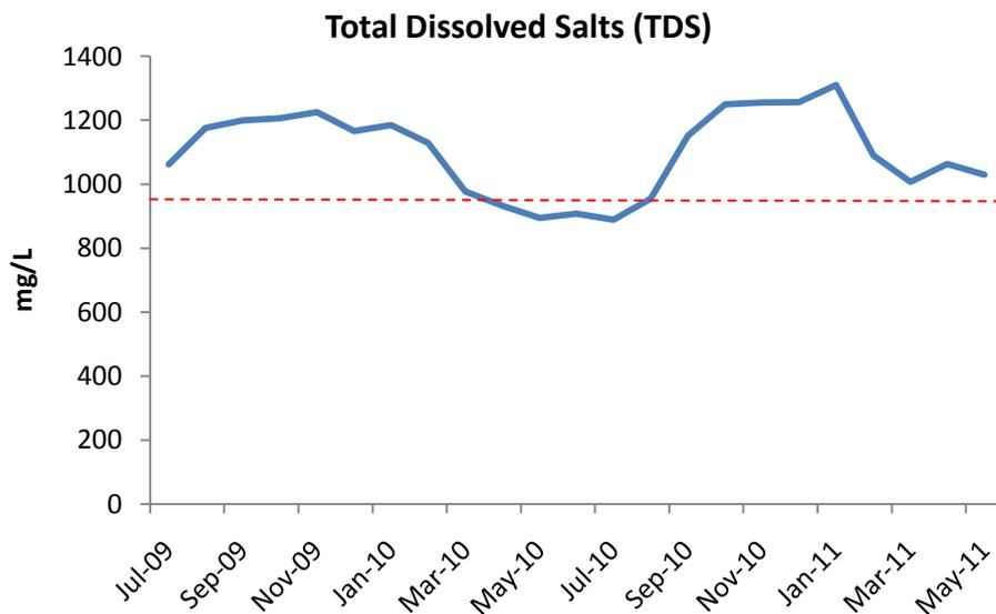
**Figure 6.** Total dissolved salts (TDS) of reclaimed water at the Bolivar wastewater treatment plant and the acceptable threshold level for almond production before foliar damage occurs (980 mg/L).
