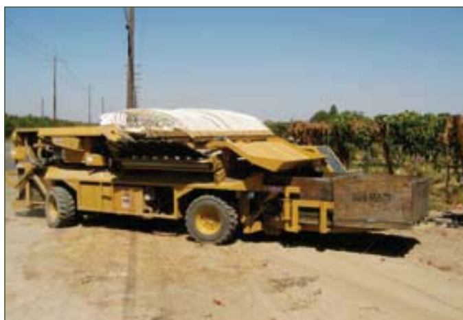
Harvester operating in overhead pergola trellis system.
