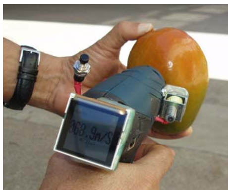
Plate 6 Acoustic velocity unit used to assess the eating soft stage of Calypso mango fruit.
