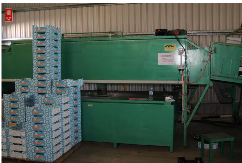
Plate 20 The hot water spray unit, with the hot fungicide spray reservoir underneath the spray tunnel.
