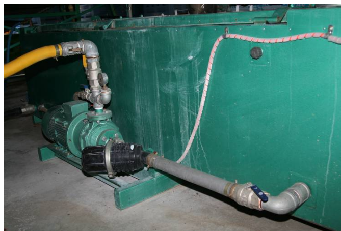
Plate 21 The pump circulating the hot fungicide from the reservoir to the spray tunnel.
