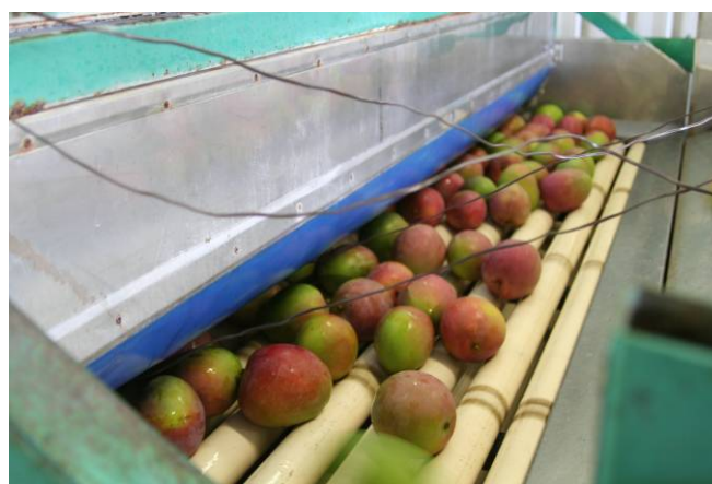
Plate 23 Thermocouple wires holding the "hypodermic" thermocouples about 2 m inside the entrance to the spray tunnel.
