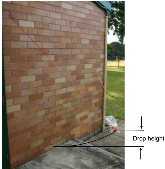
Plate 17 Method used for applying impacts to Calypso™ mango fruit.
