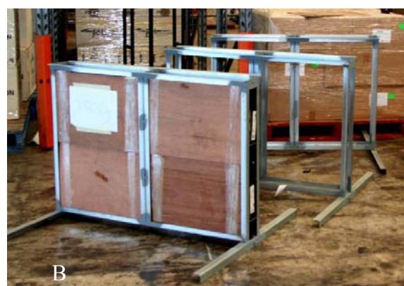
Plate 57 Tray and rack system for irradiation of B74 mango. (A) Trays were covered with ply lids with foam. (B) Trays placed vertically in racks (four trays per rack). (C) Racks placed on top of bins.
