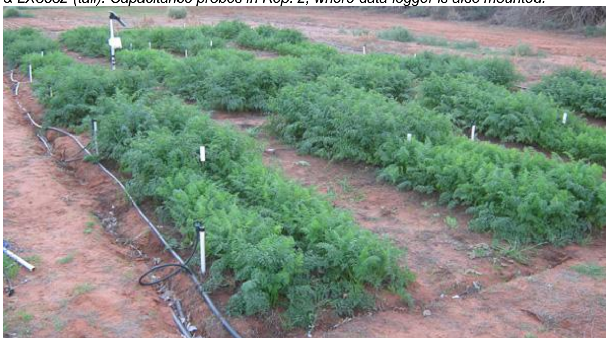
Photo 10.5 – BC0902: 115 days after planting. Alternating ends of plots for Red Hot (short) & LX3632 (tall). Capacitance probes in Rep. 2, where data logger is also mounted.
