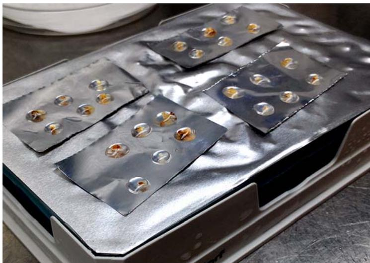
**Figure 6.** SE suspended in droplets of PVS2 on aluminium foil strips.
