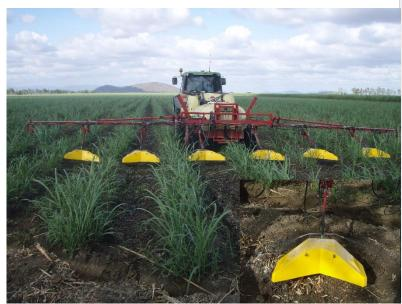
Shielded sprayer covering furrows. Inset - close up of shielded sprayer.
