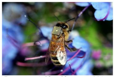
The sensors, measuring 2.5mm x 2.5mm, are currently being attached to the backs of bees in Hobart, Tasmania, prior to their release into the wild.
