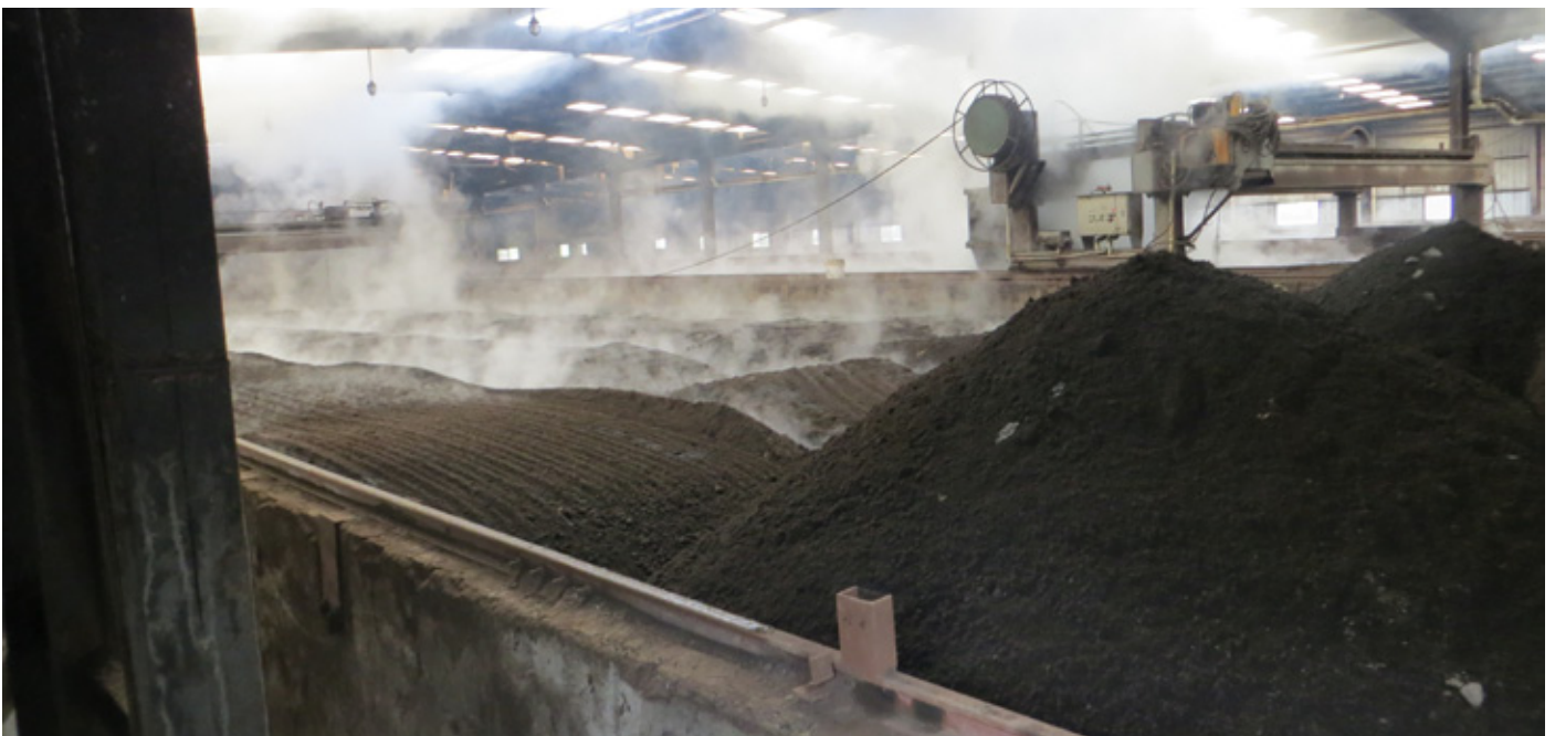
Organic fertilisers played a large role in plant nutrition in China, this is a large automated composter.
