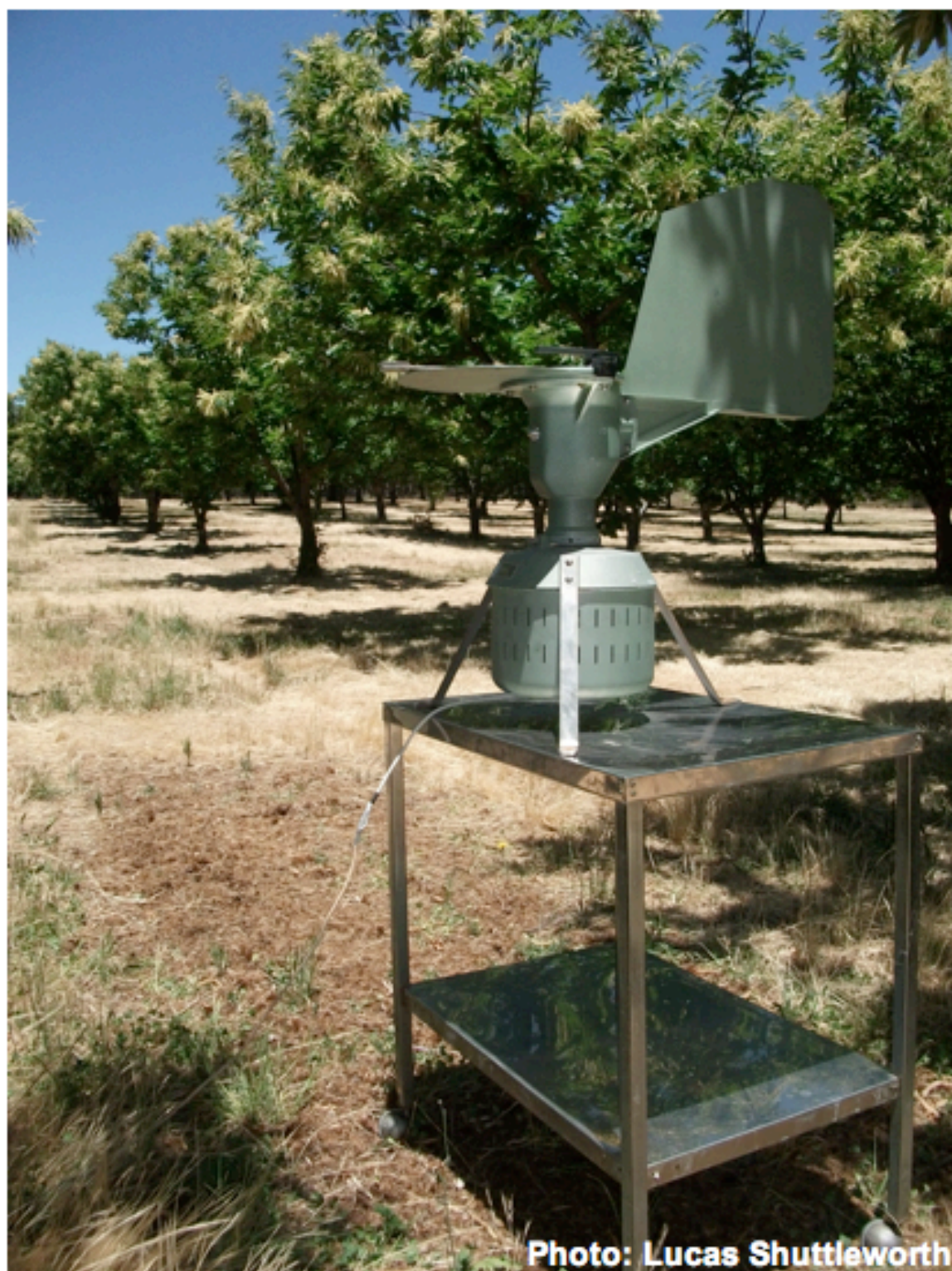
Fig. 5 Burkard Volumetric Spore-Trap set up in the chestnut orchard in Mullion Creek, NSW to capture ascospores released from decaying burrs into the orchard atmosphere during the chestnut flowering period. December 2010.
