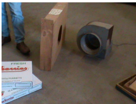
Figure 1 and 2 simple forced air cooling fan for smaller growers
