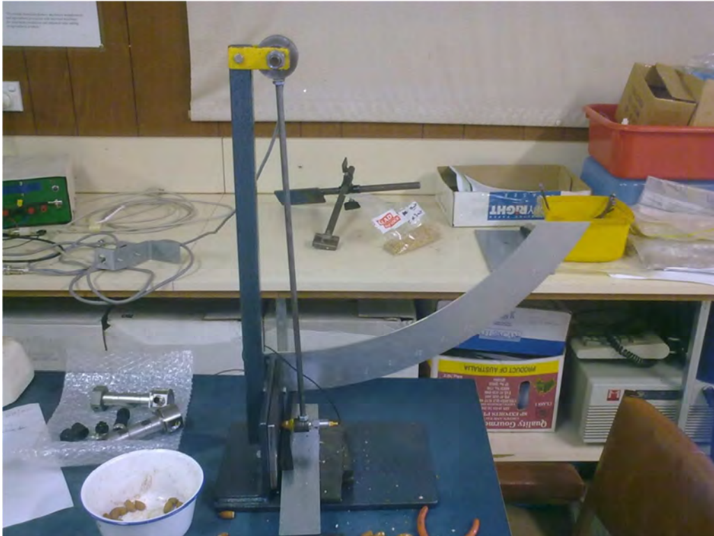
Figure 5.1 The pendulum impact tester used to create an impact against the almonds.
