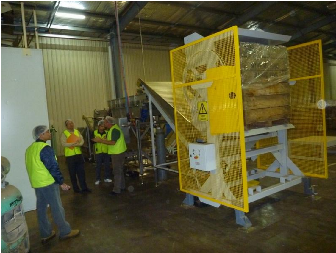
A pre-cleaning line to remove foreign material using a laser scanner.
