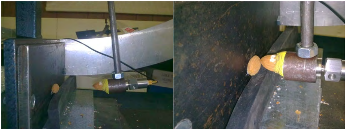
Figure 5.6 Pendulum impact tester with an almond point.
