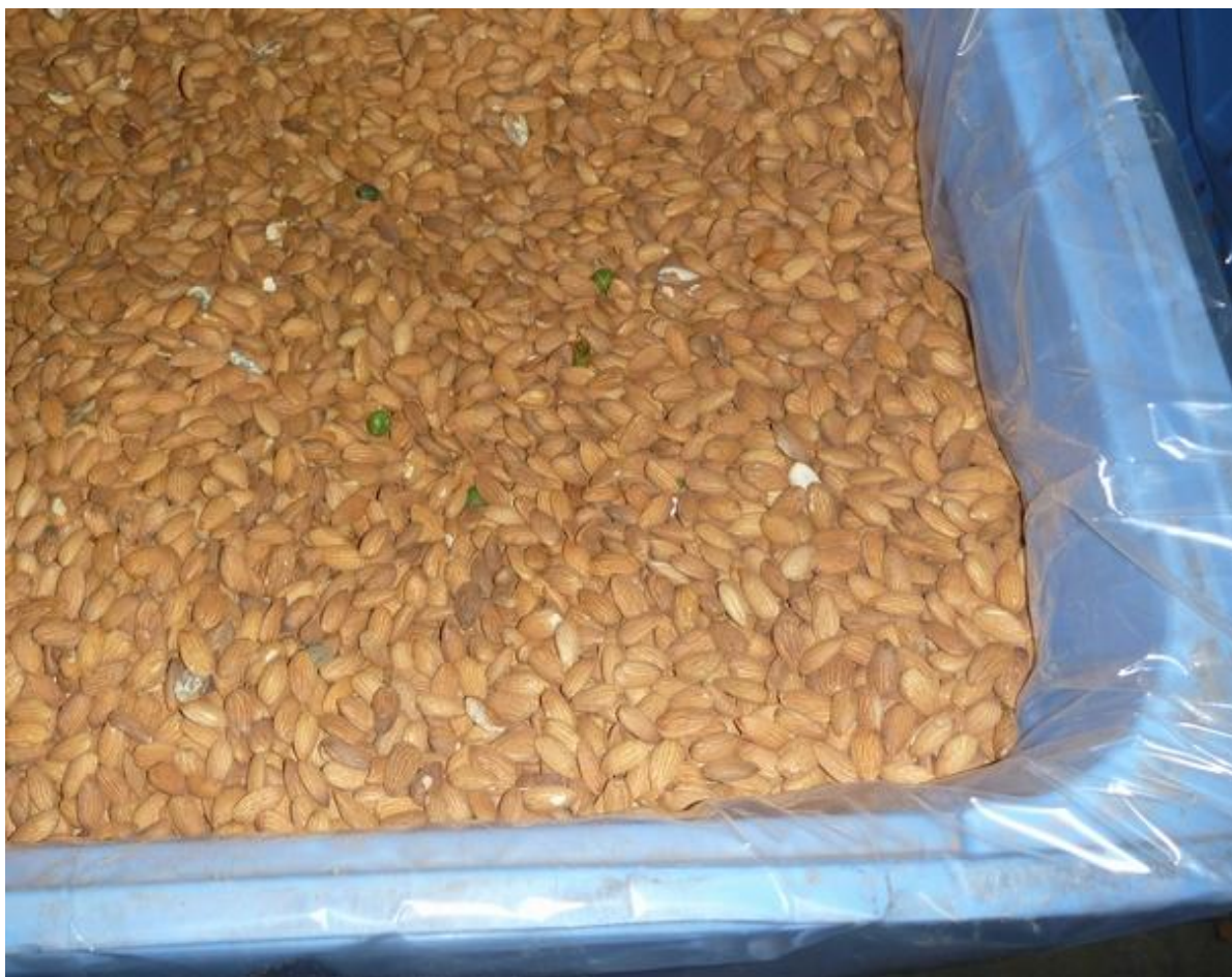
The final size graded product is not free of contaminants. Note mouldy kernels (dark) and small melons remaining.
