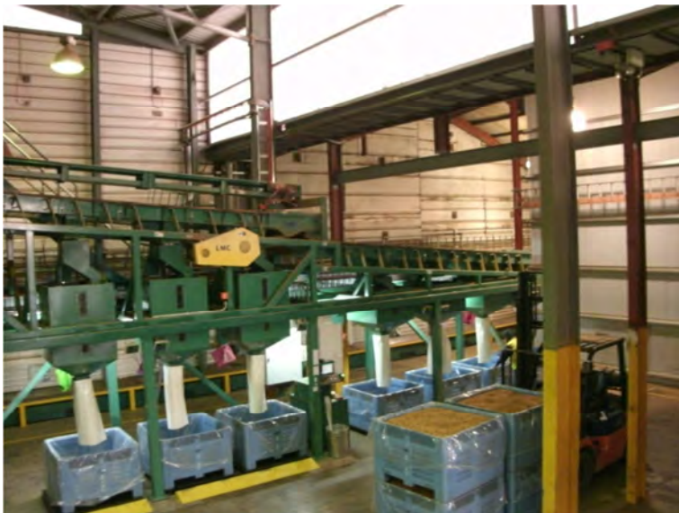
Figure 2.13 Overhead vibrating screens size grade and drop kernels into the respective bins below.
