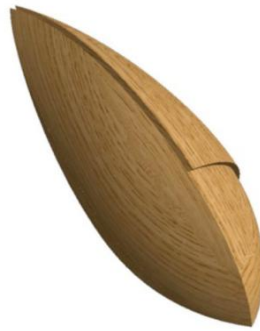
Figure 5: Second action of passing through shear rollers – cracking of shell
