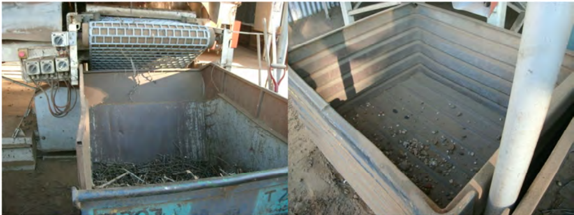
Figure 3.13 Desticker and destoner removes sticks and stones in the pre-cleaning process.
