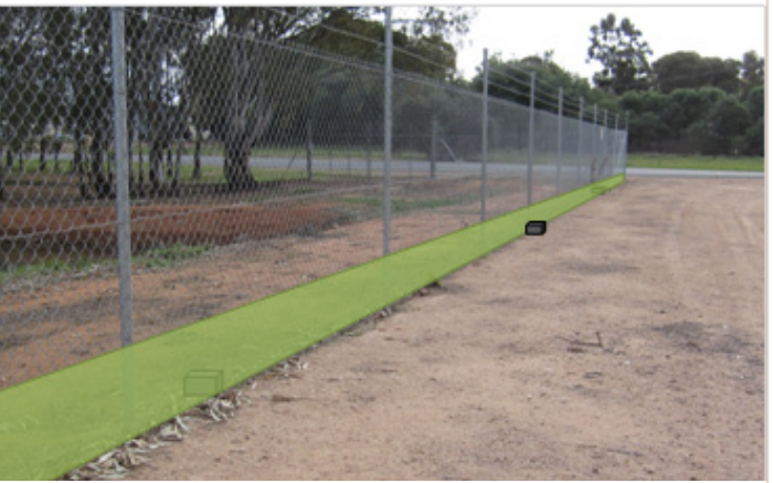
Figure 3. Example of how a drift fence could be set up along a chain link fence to help direct mice into bait stations. A 30-cm high length of shade cloth/silt fencing could be attached to the bottom of the chain link fence. The fence would guide mice into bait stations set along the bottom of the fence. Bait stations could be set alternatively on either side of the fence.
