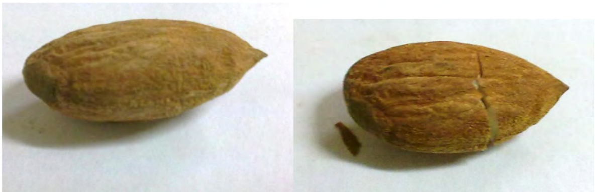
Figure 5.4 Almond kernel with no visible damage (left) shows cracks after gentle pressure was applied (right).
