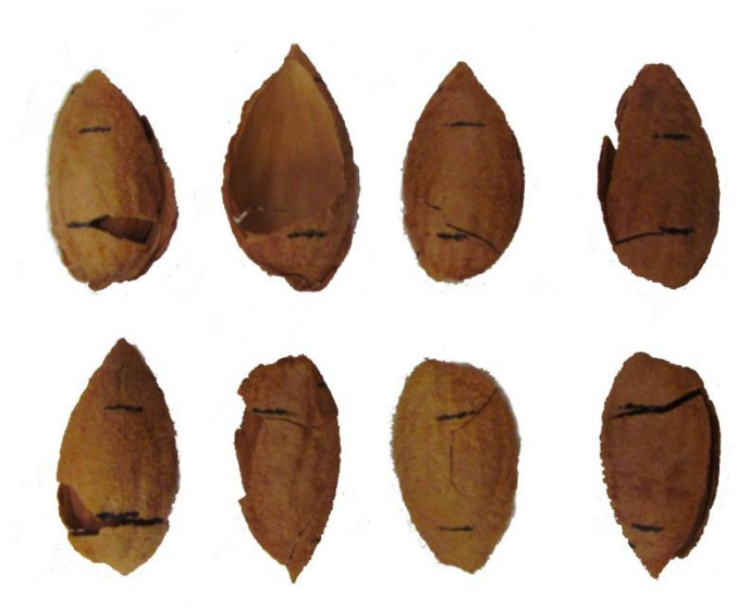
Figure 8: Results of a thickness orientation breaking test. Gap was 11.25 mm
