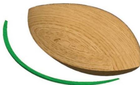
Figure 4: First action of passing through shear rollers – removal of tongue. The green item highlight the tongue removed.
