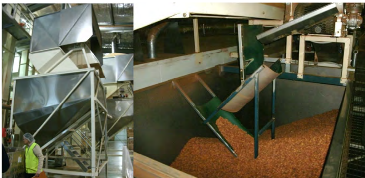
Figure 3.4 Hopper for loading almond kernels into the color sorters (left). Cascades at Riverland Almonds (right).
