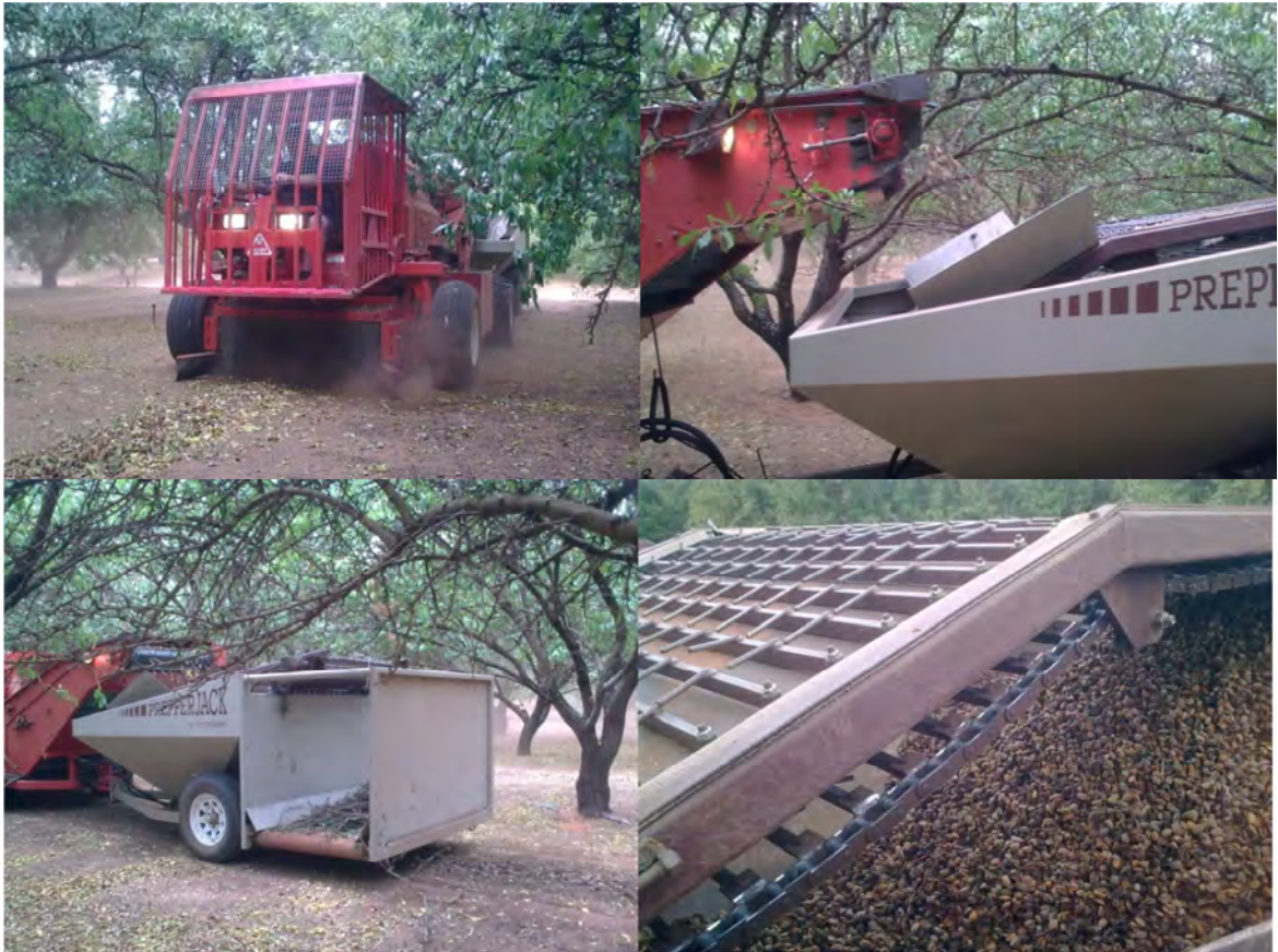
Figure 2.9 A pickup with an optional integrated desticker in operation.
