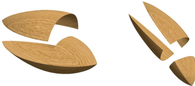
Figure 6: Final breaking of the shell in one of 2 ways. Either single sided or double sided cracking
