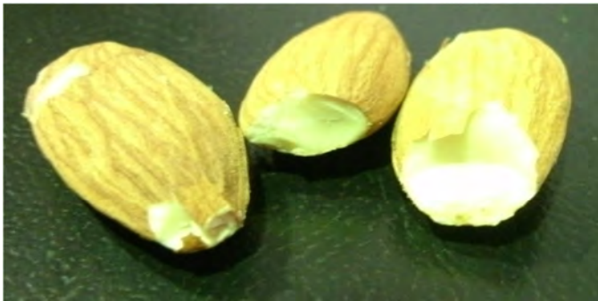
Figure 5.12 Almond kernels broken at 19m/s.
