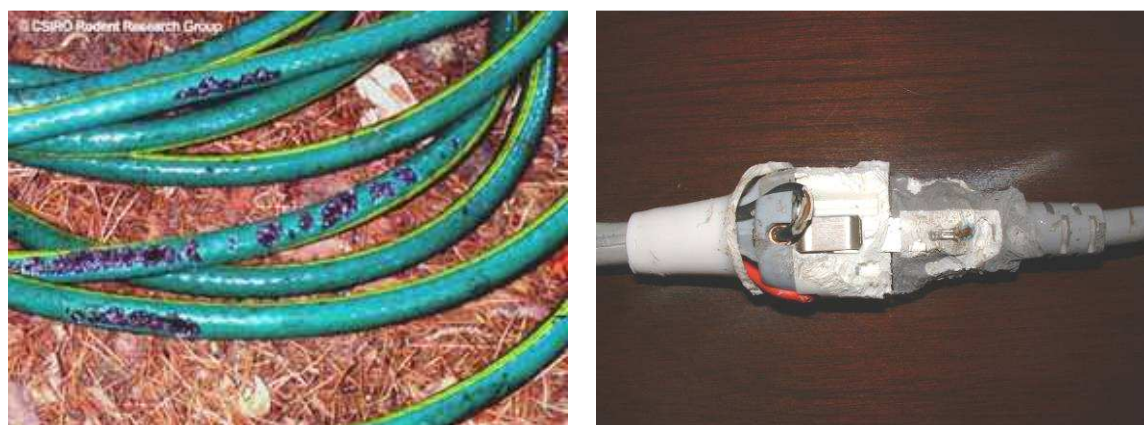
Figure 1. Left: Rodent gnawing on a domestic garden hose. Right: Rodent damage to an electric power lead (source: http://www.greenpest.com.au/rodents.htm#Mice ).
