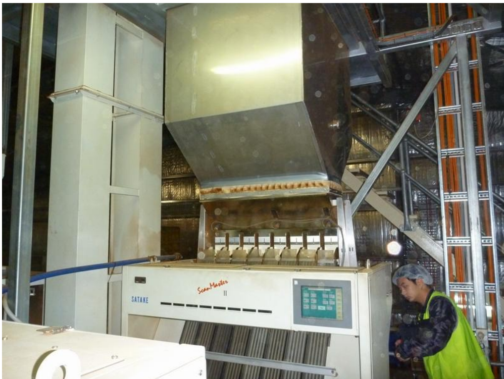
A pre-cleaning line to remove foreign material using a laser scanner.
