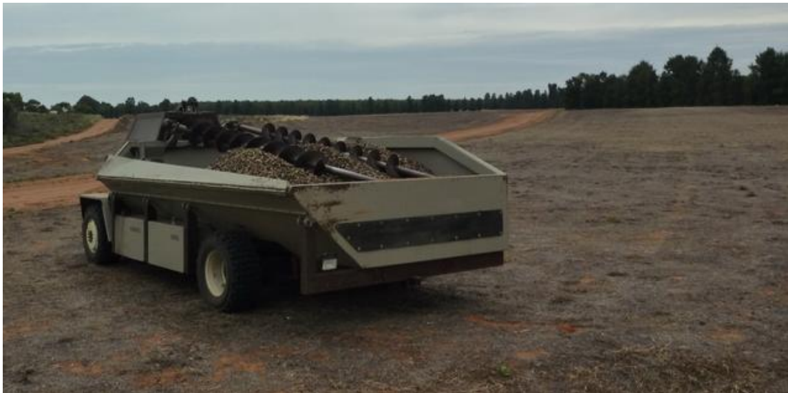
Haul out of almonds (note rear bumper which pushes against a lever on pickup to start transfer of almonds into the haul out vehicle).
