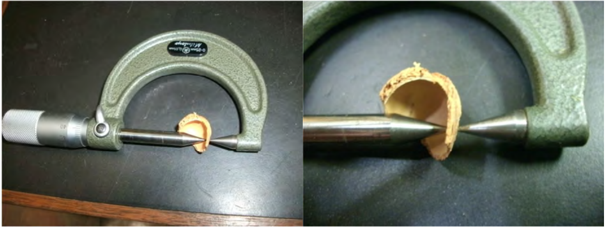
Figure 4.15 Measuring the thickness of the almond shell with a point micrometer.
