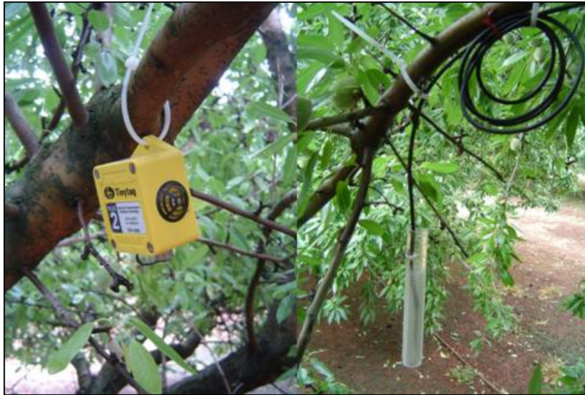
Photo 1 : Relative humidity, temperature and leaf wetness sensors
