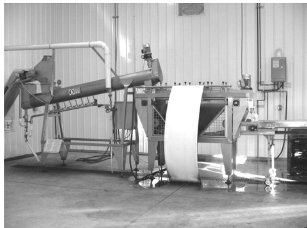
Chestnut peeler showing (L to R) steamer unit, brush unit and inspection table
