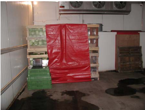
Figure 9.1.2c. Conventional forced air cooling of prototype bins.
