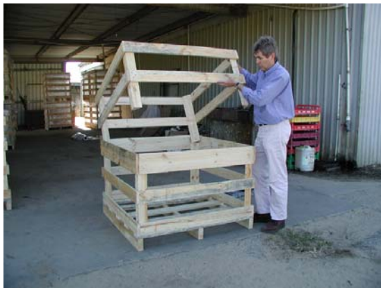
Figures 9.3.6a. The two halves of the modular bin being fitted together.
